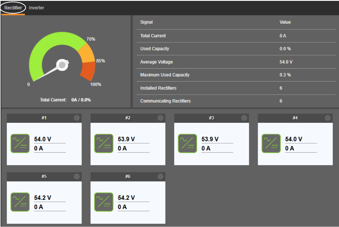
Figure 5.6 Rectifier Device Group Status Page Tab
