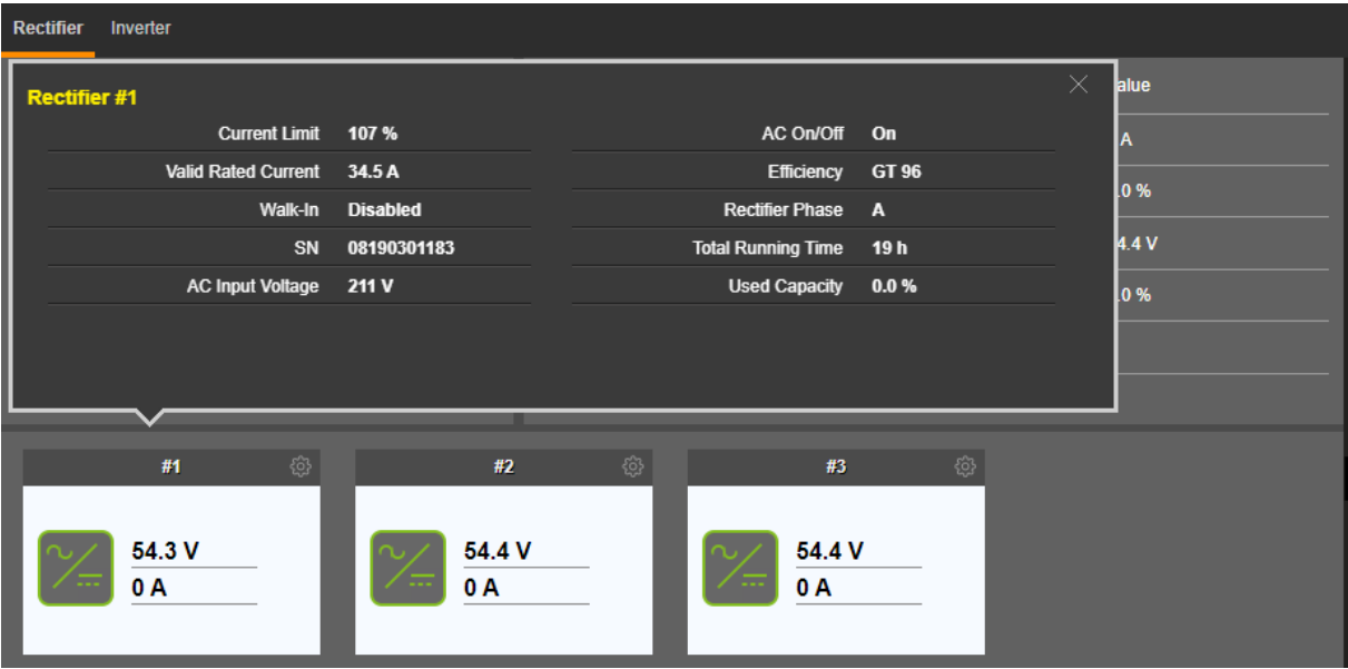
Figure 5.7 Individual Rectifier Status Page
