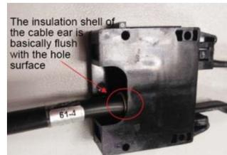
Figure 3-7 Cable flush
