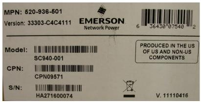
On your switch unit, locate the white Emerson Network Power sticker. On the right-hand side of the label, under the Emerson logo, the unit serial number (S/N) will be indicated with a combination of letters and/or numbers listed below a bar code. For example, the serial number is HA27160074 as indicated in the following graphic.
