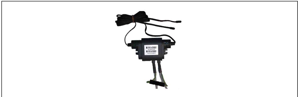
Figure 12.10 CANbus and Ground Connection on 2T Sensor
