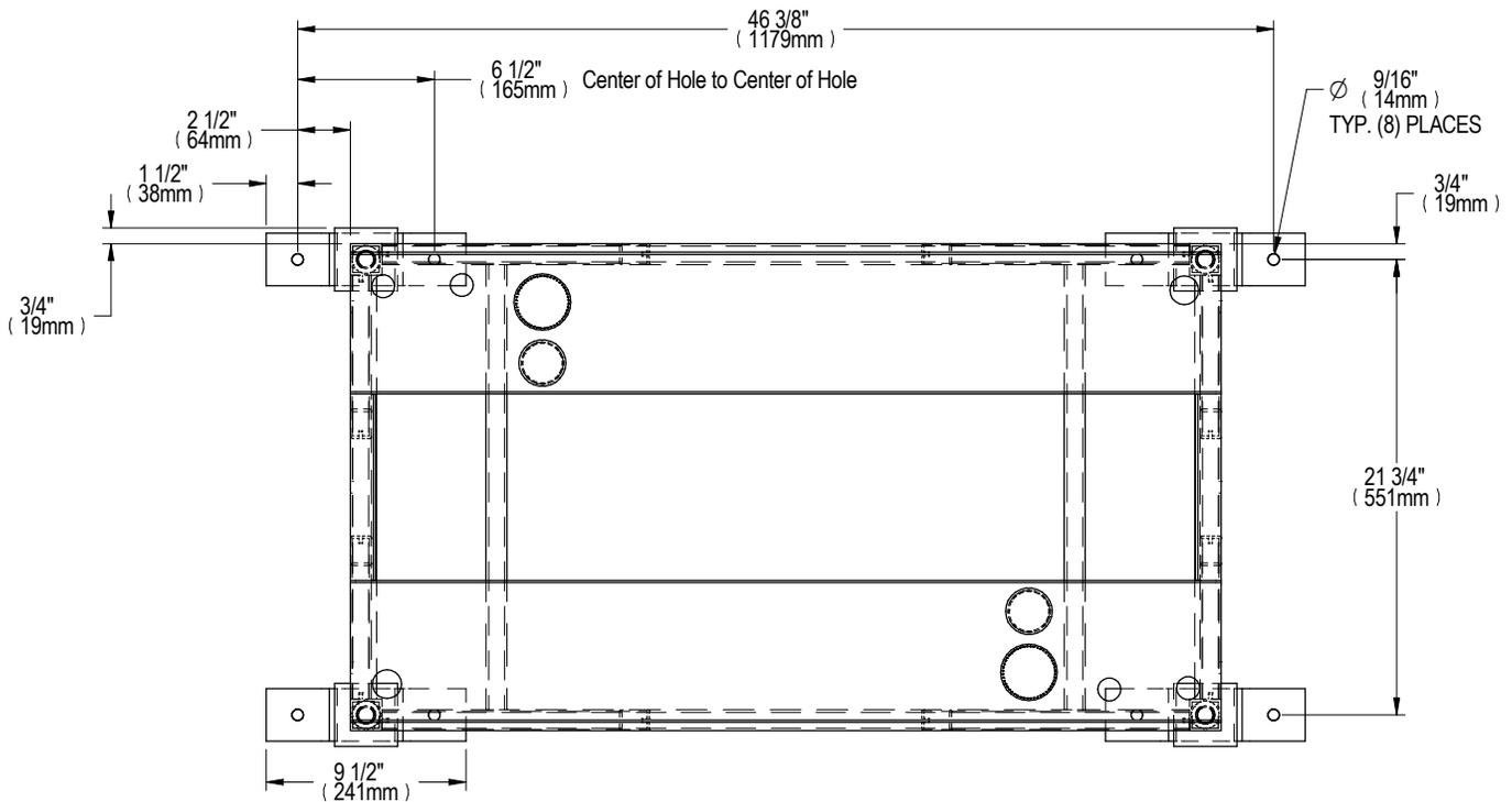
FLOORSTAND ANCHORING DIMENSIONS TOP VIEW
