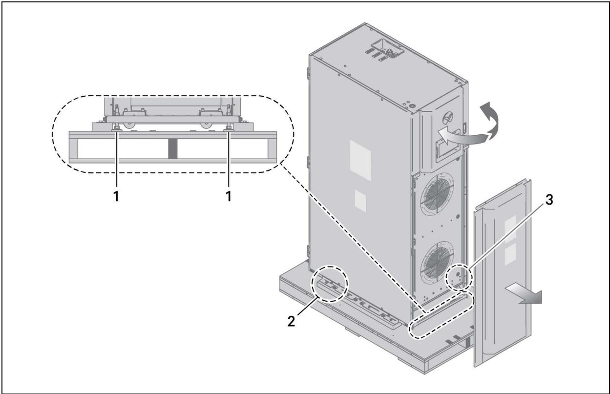
2. Lower the four stabilizer feet to make contact with pallet deck using a 3/8-inch (10 mm) socket drive or wrench.
