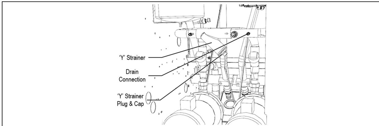
**NOTE:** The XDU must be shut down to remove and clean the Y-strainer. This will stop cooling of the connected load. Take all necessary steps to prevent damage to the load.
