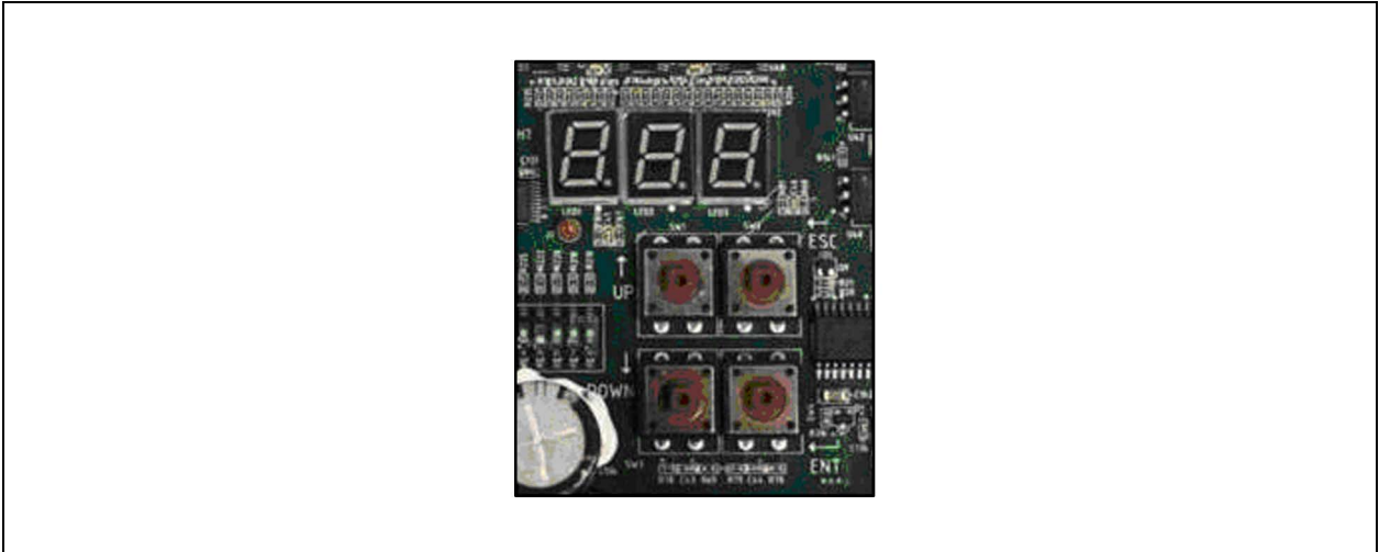
Figure 10.6 Control Board HMI
