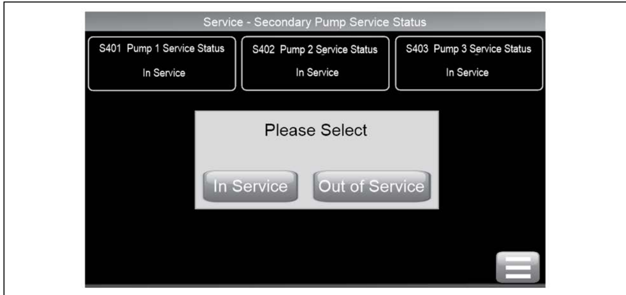
Figure 7.4 Service - Secondary Pump Service Status
