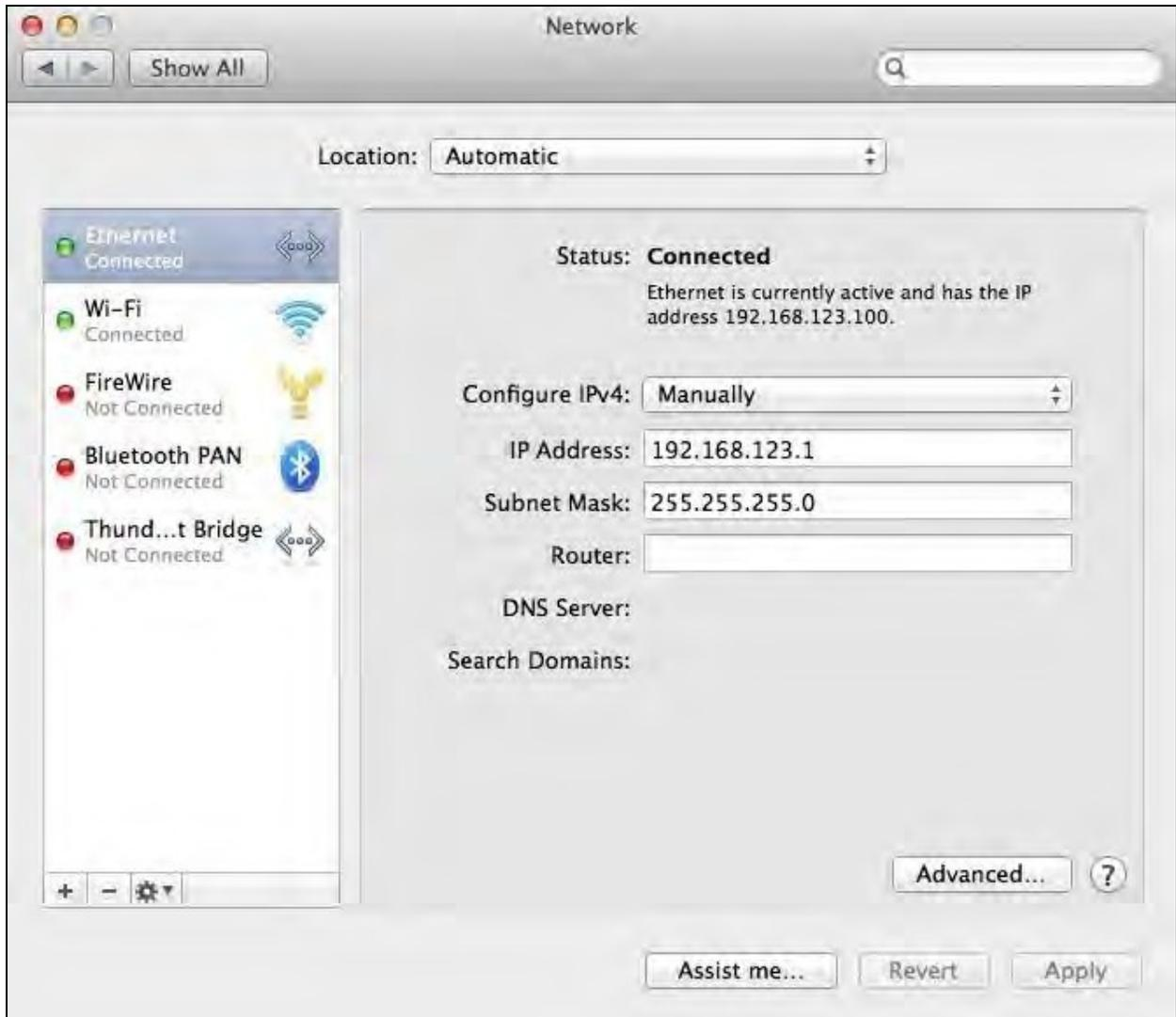
2. Ensure *ETHERNET* is highlighted on the left side of the NIC window. In most cases, there will be one *ETHERNET* entry on a Mac. Write down the current settings so you can restore them to normal after you have completed the setup procedure.
