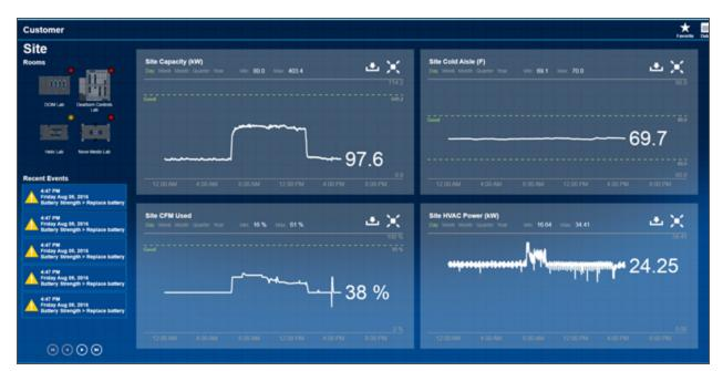
Figure 6.6 iCOM-S Software User Interface With Site Information
