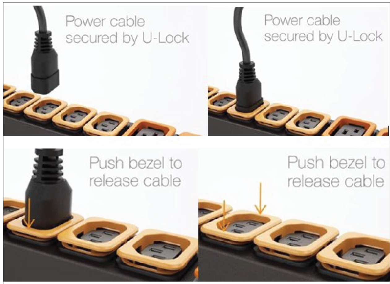
Figure 3.15 U-Lock Cord Retention Operation
