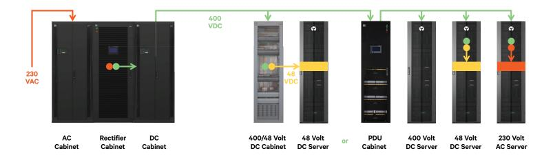
The Vertiv™ NetSure™ HVT solution includes all of the components required for your 400V HVDC power site including a rectifier cabinet, DC distribution cabinet, optional AC distribution cabinet, PDU cabinet, as well as supporting control and monitoring devices.
