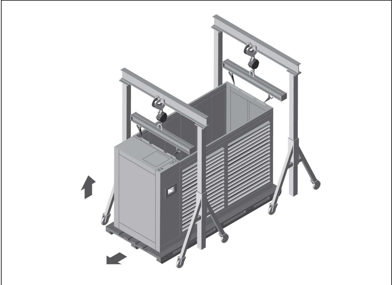
5. Use the rigging equipment to move the unit to the final installation location, see **Figure 4.6** below .
