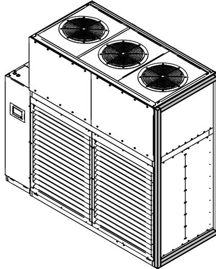
Gasketing shown is for pictorial purposes only to show edges of unit that require gap sealing. Gasketing and method to be provided and applied by others in the field.
