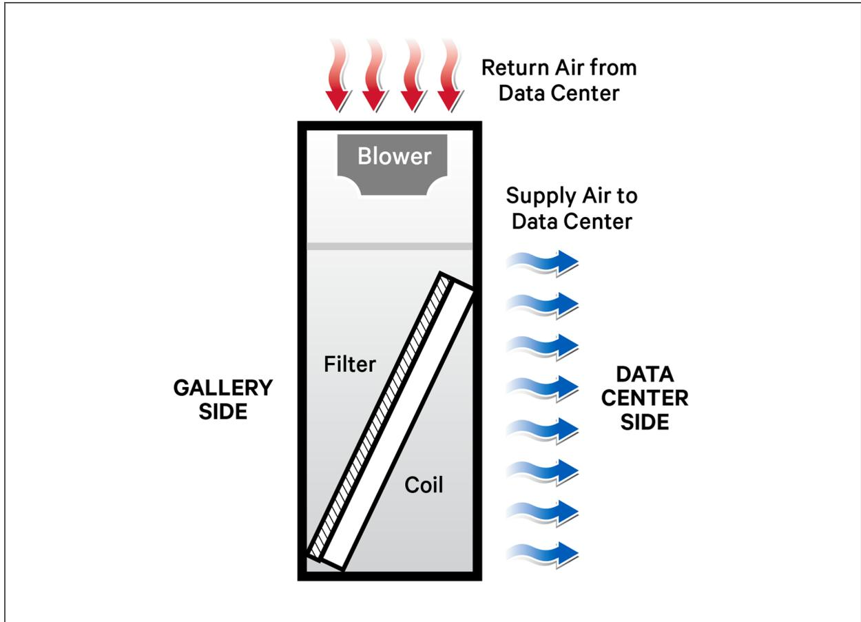
Figure 1.2 Downflow, horizontal-discharge blower configurations with EC fans on a floor stand
