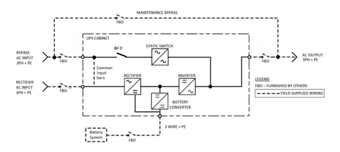
**Note:** 1250 kVA ratings are shipped without single input links connecting the rectifier and bypass AC input phase bus bars. Links can be ordered if needed.
