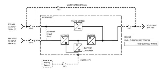
**Note:** 1250 kVA ratings are shipped without single input links connecting the rectifier and bypass AC input phase bus bars. Links can be ordered if needed.
