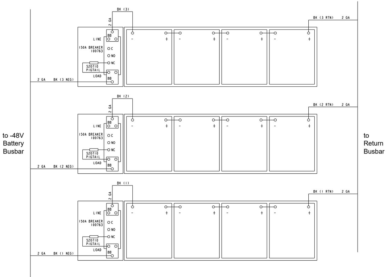
**Figure 3.7 Battery Tray Wiring Diagram (582127000203 and 582127000503 only)**
