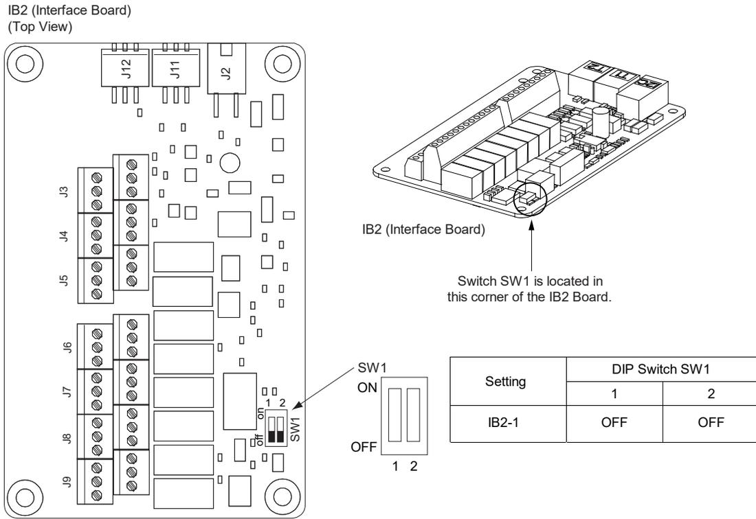
**Figure 4.4 Optional EIB Controller Extended Interface Board Switch Location and Setting**
