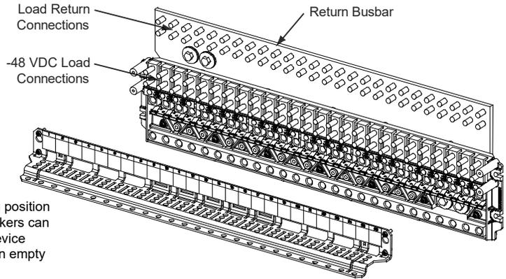
Caution: A 100 A circuit breaker or fuse SHALL HAVE an empty mounting position between it and any other overcurrent protective device. 100 A circuit breakers can be used without a space provided the continuous current in each 100 A device does not exceed 64 A. A 175 A or greater circuit breaker SHALL HAVE an empty mounting position between it and any other overcurrent protective device.
