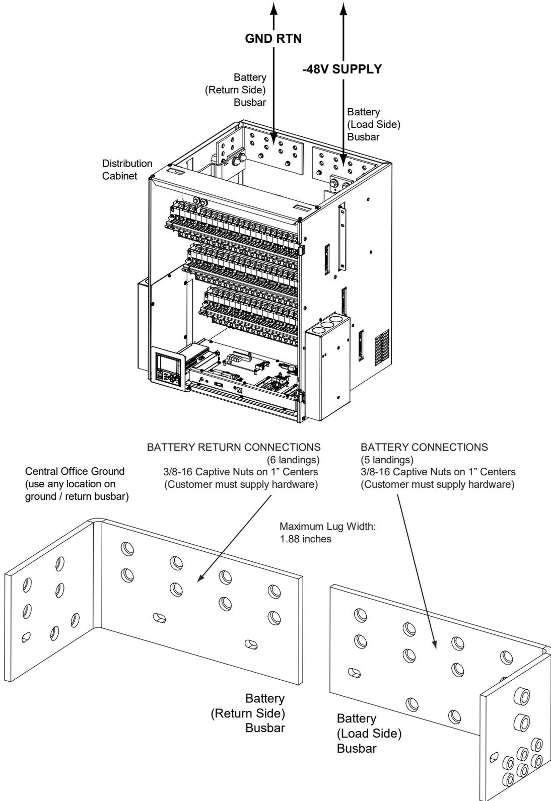
**Figure 5.15 Battery Busbar Dimensions**
