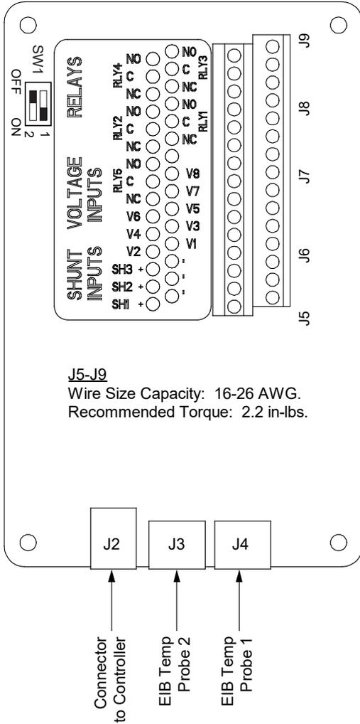
Schematic Diagram of EIB Board
