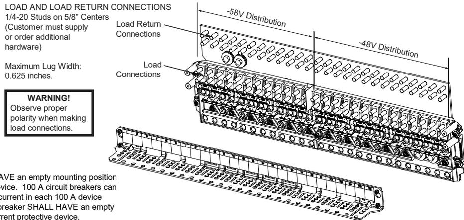
Caution: A 100 A circuit breaker or fuse SHALL HAVE an empty mounting position between it and any other overcurrent protective device. 100 A circuit breakers can be used without a space provided the continuous current in each 100 A device does not exceed 64 A. A 175 A or greater circuit breaker SHALL HAVE an empty mounting position between it and any other overcurrent protective device.
