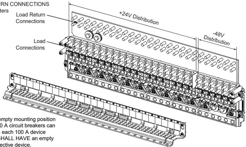
Caution: A 100 A circuit breaker or fuse SHALL HAVE an empty mounting position between it and any other overcurrent protective device. 100 A circuit breakers can be used without a space provided the continuous current in each 100 A device does not exceed 64 A. A 175 A or greater circuit breaker SHALL HAVE an empty mounting position between it and any other overcurrent protective device.
