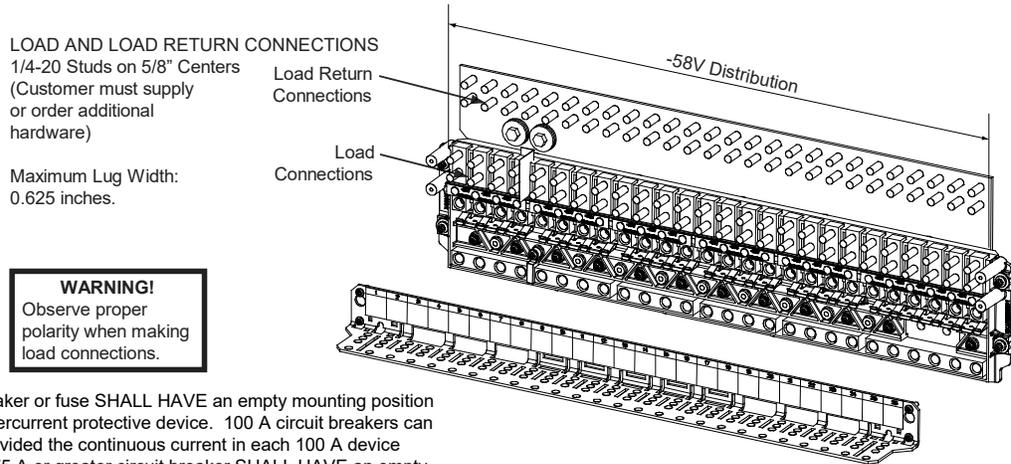
Caution: A 100 A circuit breaker or fuse SHALL HAVE an empty mounting position between it and any other overcurrent protective device. 100 A circuit breakers can be used without a space provided the continuous current in each 100 A device does not exceed 64 A. A 175 A or greater circuit breaker SHALL HAVE an empty mounting position between it and any other overcurrent protective device.
