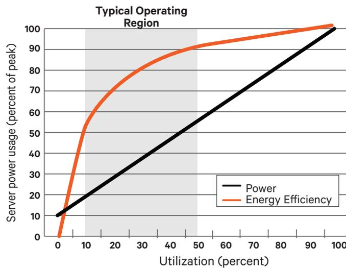
Source: Hölzle, 2017. Note: In a more energy-proportional server (red line) the power efficiency is more than 80% of peak value for utilization levels of 30% or more with efficiency remaining above 50% for utilization levels as low as 10%.
