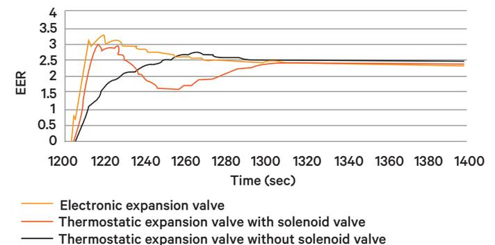
Note: Values measured during testing with the EEV are always higher than the EER values measured using the TXV, with or without a solenoid valve. This higher energy efficiency is ensured by the EEV's capability to optimize the control of refrigerant flow in the evaporator, thus limiting the delivery of liquid into the compressor.
