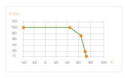
Output Power vs. Temperature at 264 ≥ Vin ≥ 176 VAC
