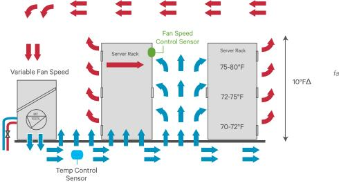
Figure 6: Liebert® iCOM™ fan speed control sensors on the server racks match airflow to the conditions at the servers
