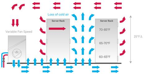
Figure 4: The fan speed is too high in this data center, resulting in wasted energy from the loss of cold air.
