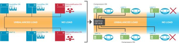
Figure 1: System-level control after optimization reduces conflict between room air conditioning units operating in different zones in the data center.
