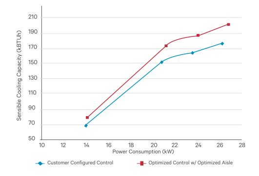
Figure 2: Over time, utilizing the Liebert iCOM control system with an optimized aisle configuration and control setting improves efficiency. Having those controls optimized properly by a factory-trained technician provides more capacity with similar levels of power consumption than if those controls were configured by the customer alone.
