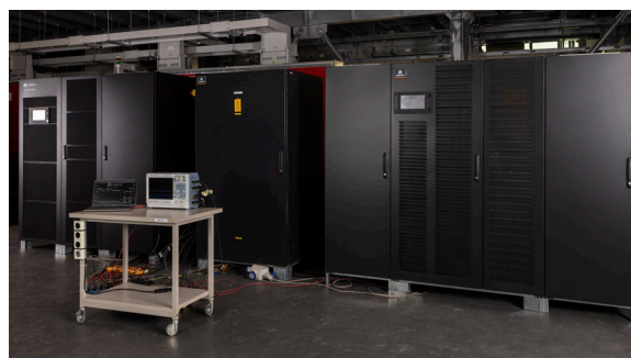
Vertiv™ PowerUPS 9000 paired with AI load simulator for advanced power testing
