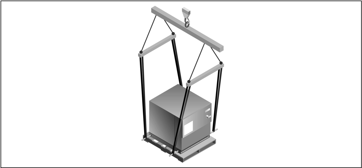
Figure 5.3 Typical Sling Arrangement for Lifting Unit
