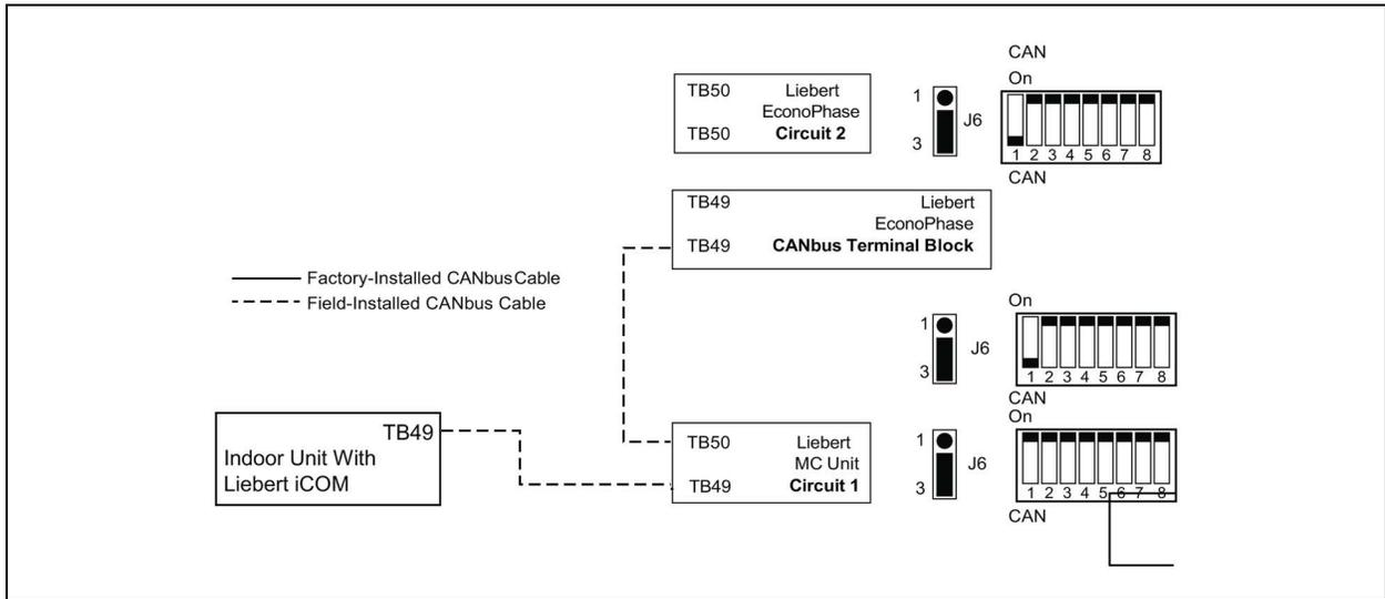
Figure 7.2 CANbus Cable Connections for Dual Circuit System, PR080 to PR250
