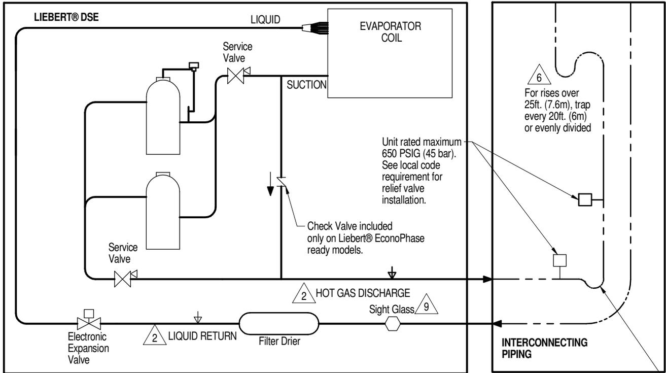
FACTORY REFRIGERANT PIPING      FIELD PIPING      SERVICE/SCHRADER (ACCESS) CONNECTION, NO VALVE CORE.      SERVICE/SCHRADER (ACCESS) CONNECTION, WITH VALVE CORE.     6 Trap at base of risers over 5ft. (1.5m)
