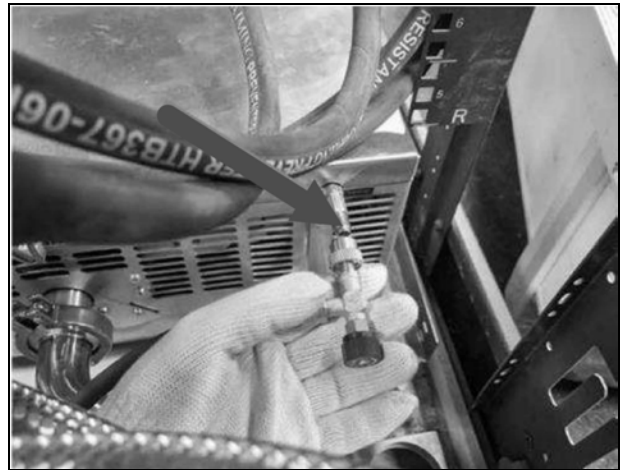
Figure 5.3 Depressing the Schrader Valve
