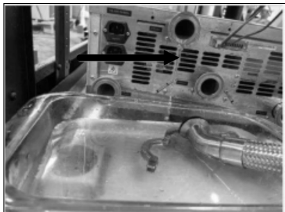
Figure 5.5 Fluid Draining, Removing Secondary Hygienic Fitting
