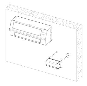
4. Use two (2) M4x50mm expansion bolts (not included) in the perforations for better grip of the fastening method. Place the bolts, leaving a space between the wall and the bolts head of at least the thickness of the sheet.
