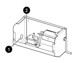
9. Redirect the pump outlet / drain hose (B) towards the location where the drained water wants to be taken (hose internal dia.: 1/4" / 6mm). Don't forget to install the anti-siphon device in the same direction of the water flow.
