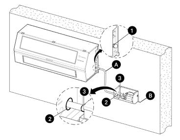
and the other end to the condensate pump. Finally, use the metal clamp to secure the drain pipe A in place.
