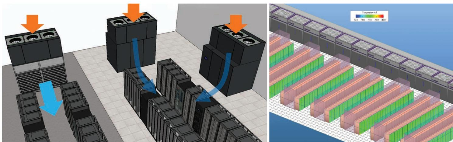
*The Liebert® DSE 250-265kW provides a high level of application flexibility. Its split-system design support situations where outdoor packaged systems are impractical. Multiple airflow configurations provide flexibility for raised-floor and slab-floor environments. Installing the units side by side creates a wall of cooling configuration which saves white space and provide access to the unit from outside the white space.*
