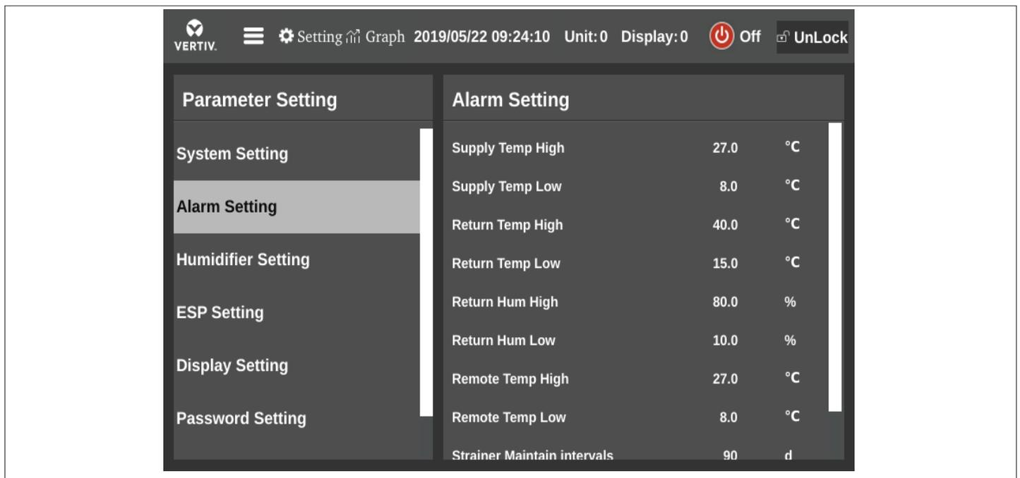
**Figure 3-13 Alarm Setting Parameters**
