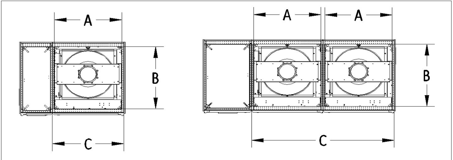
**Figure 2-16 The Position of Air Outlet on Top Cover Upflow Unit**
