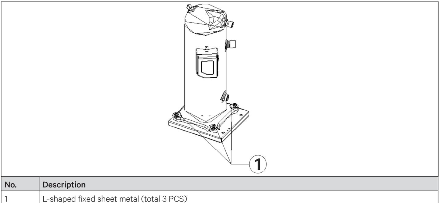
**Figure 2-28 Position of “L” Shape Fixing Plate**
