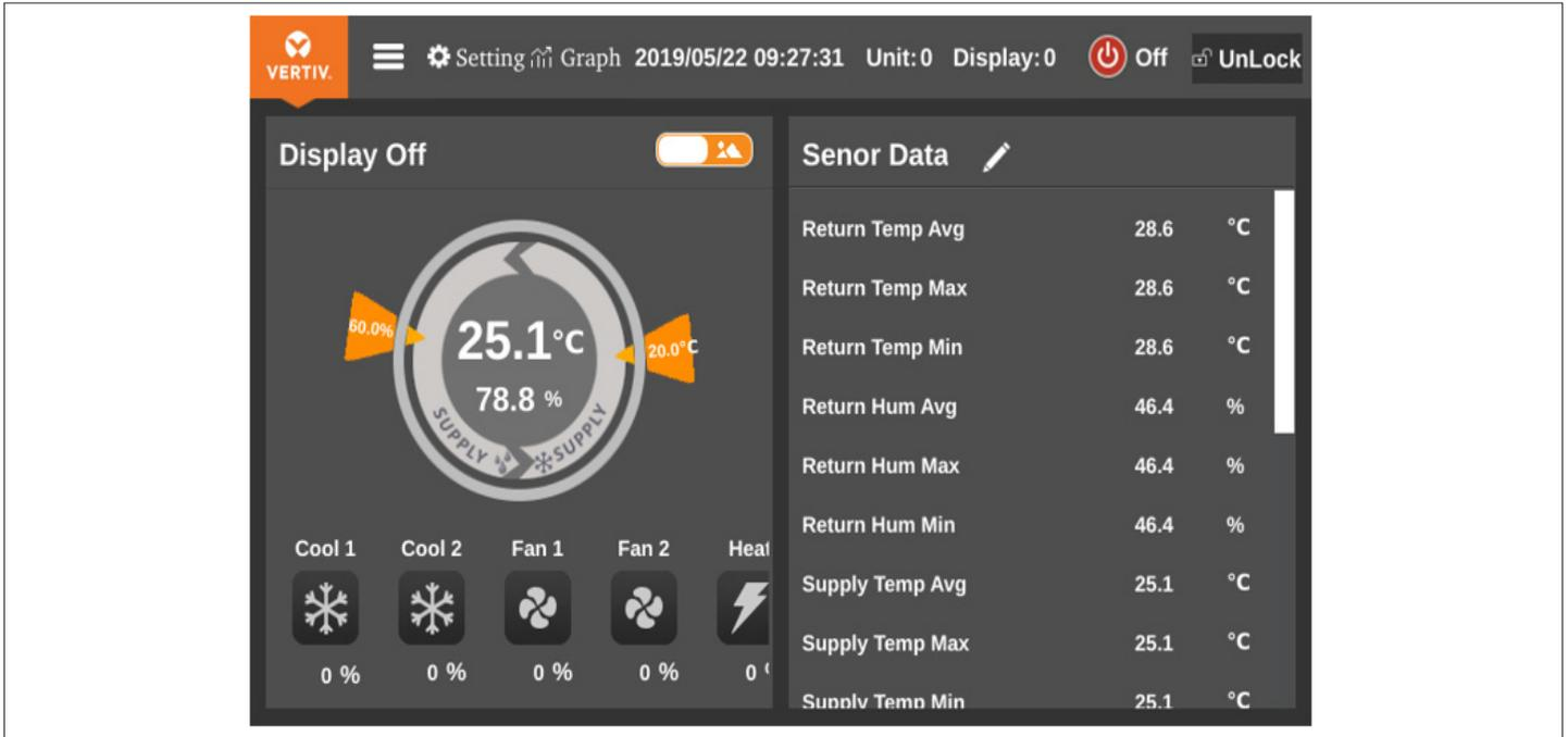
Figure 3-5 Real-time Sensor Data Parameter List - Unlocked
