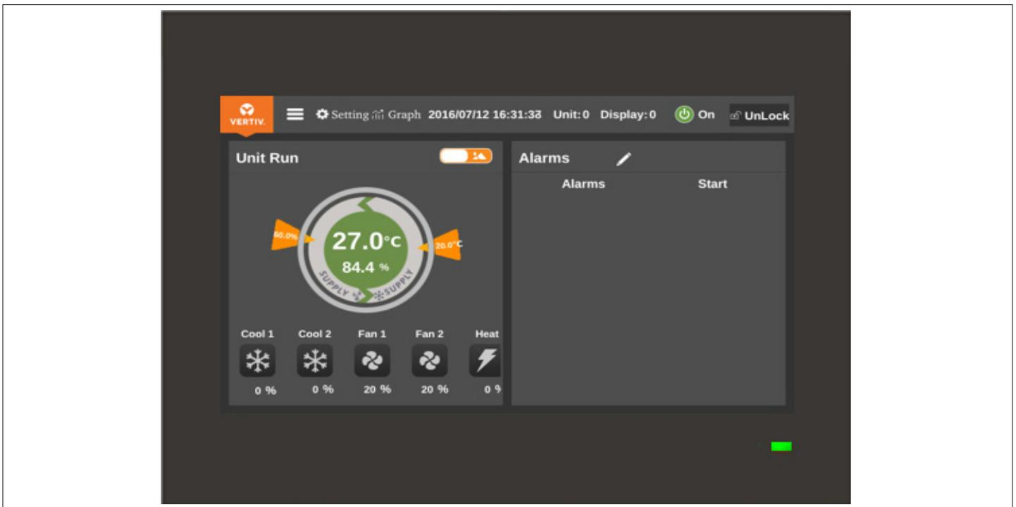
**Figure 3-1 HMI Screen Display Panel Main Interface**
