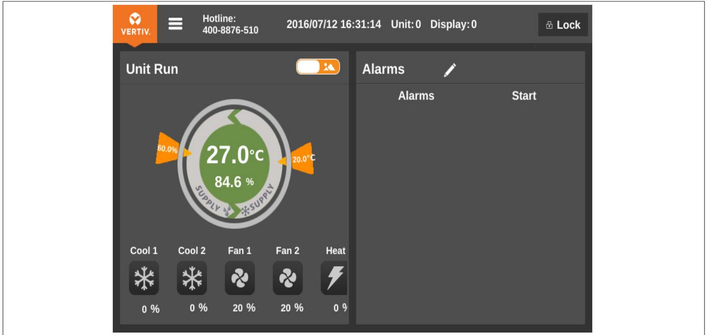
**Figure 3-3 Color Display Screen – Locked**
