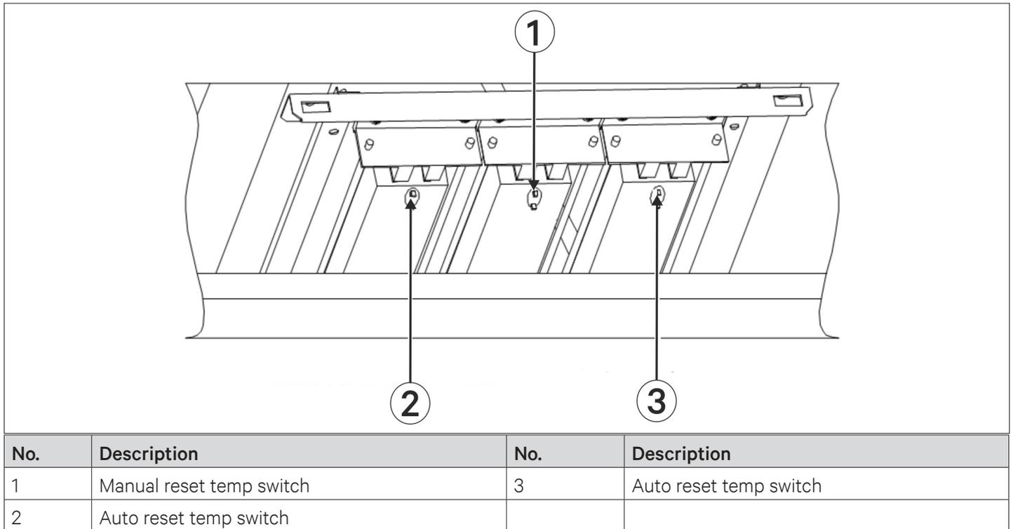
**Figure 4-2 PTC Electrical Reheater**
