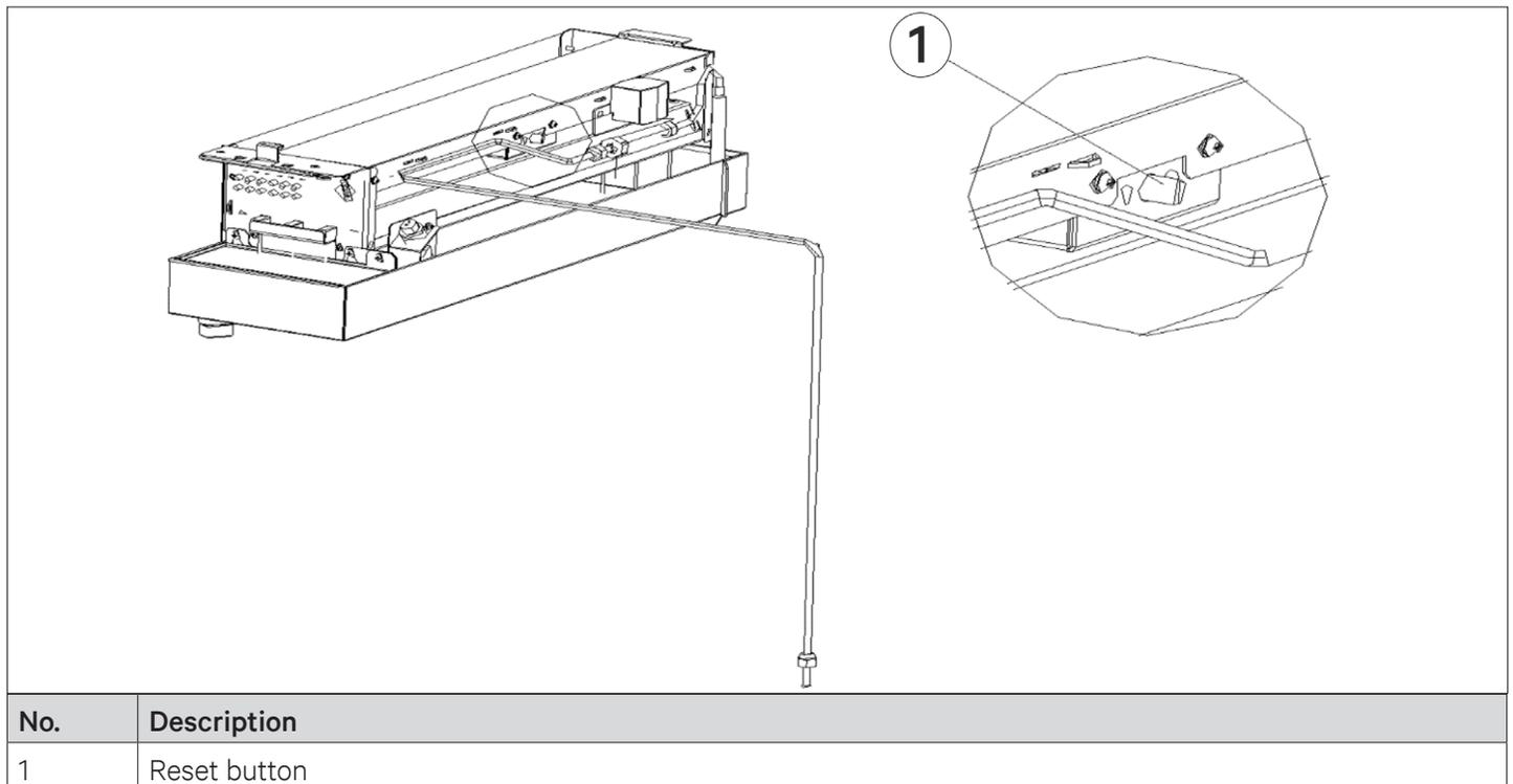
**Figure 5-1 Infrared Humidifier Reset Button**
