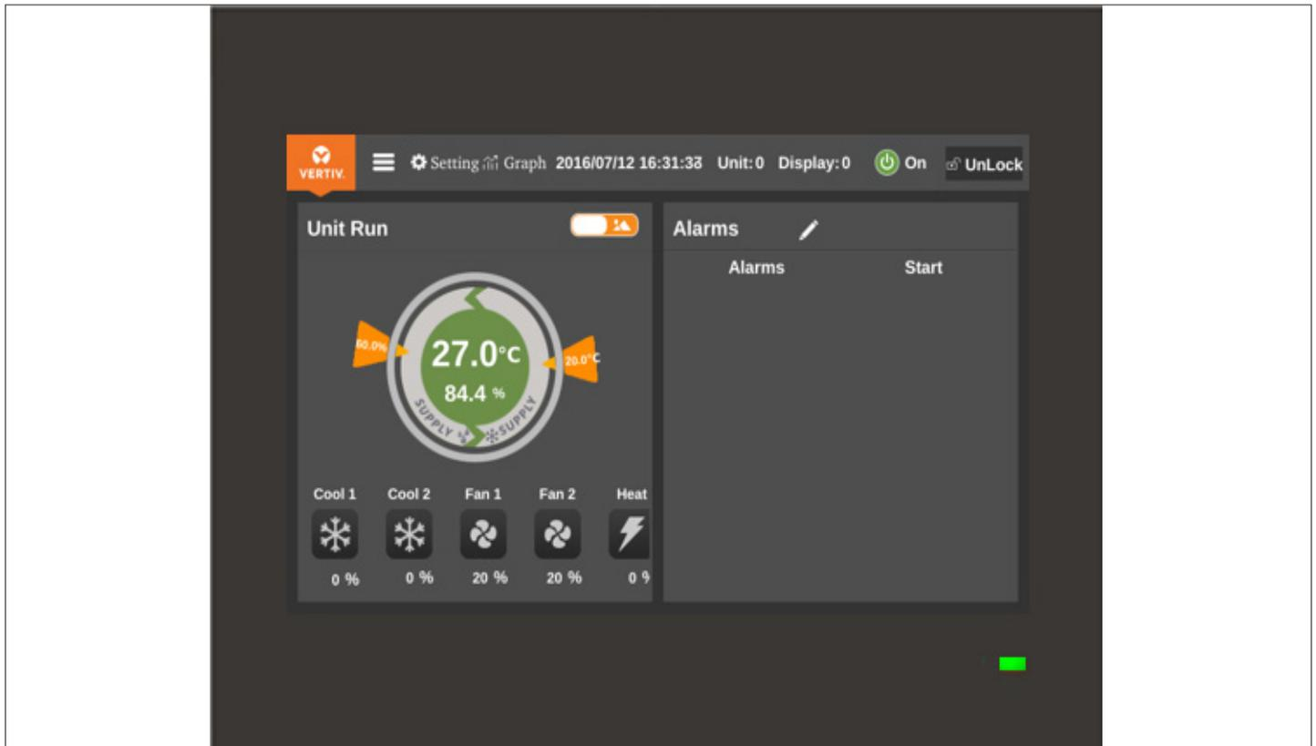
**Figure 3-4 Color Display Screen – Unlocked**
