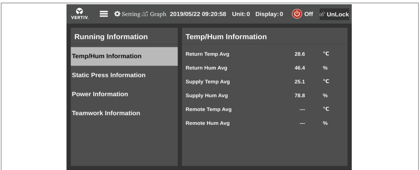
*Figure 3-19 Temperature and Humidity Status*
