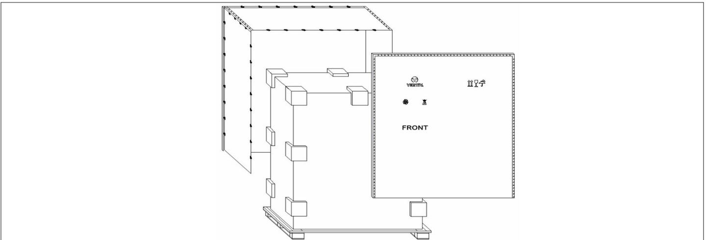
**Figure 2-5 Removing Side Panel and Top Cover**
