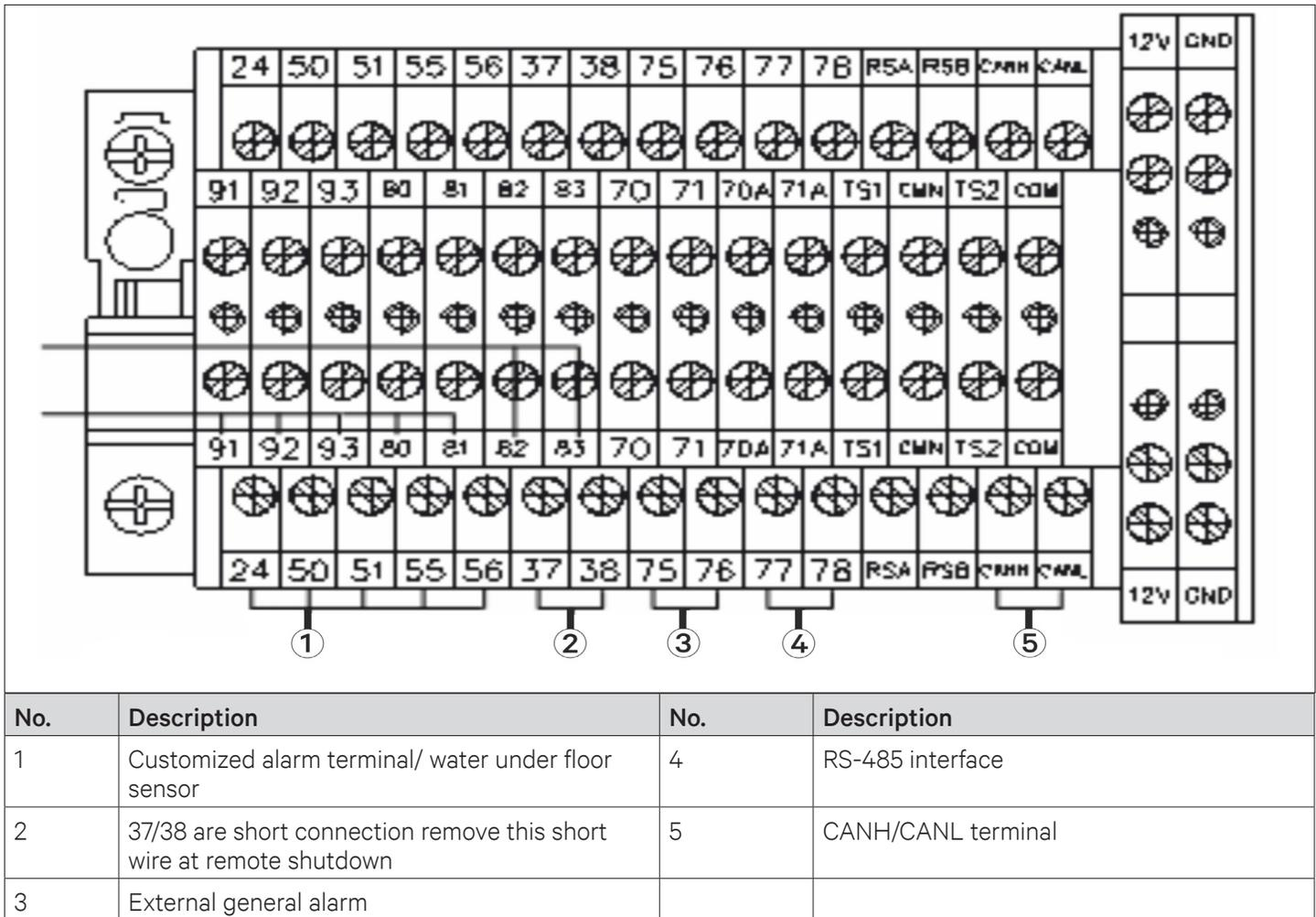
**Figure 2-32 Enlarged View of Terminal Block**
