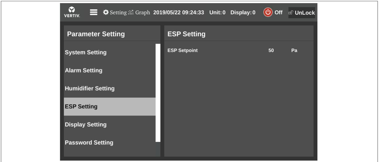
**Figure 3-16 External Static Pressure Settings**
