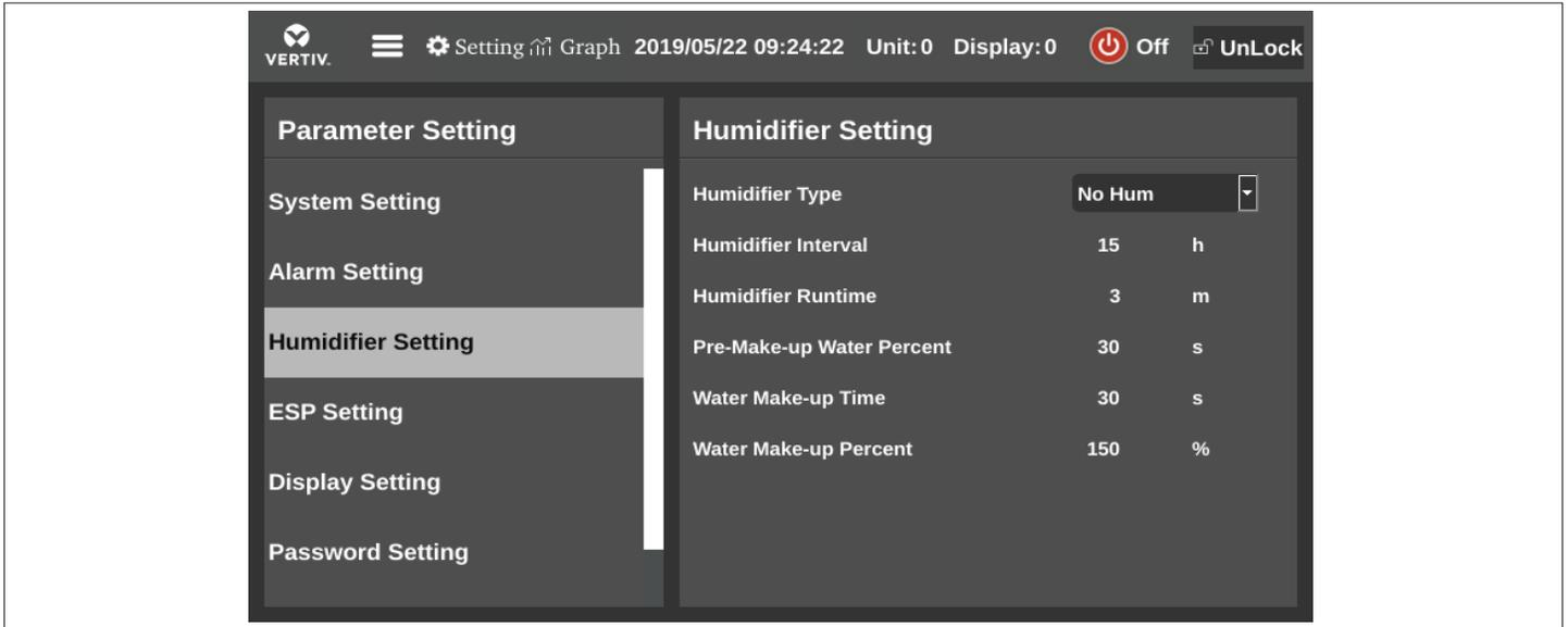
**Figure 3-14 Humidifier Setting Parameters**
