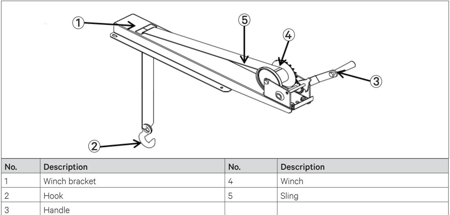
**Figure 2-24 Fan Elevator Assembly (Winch mode)**
