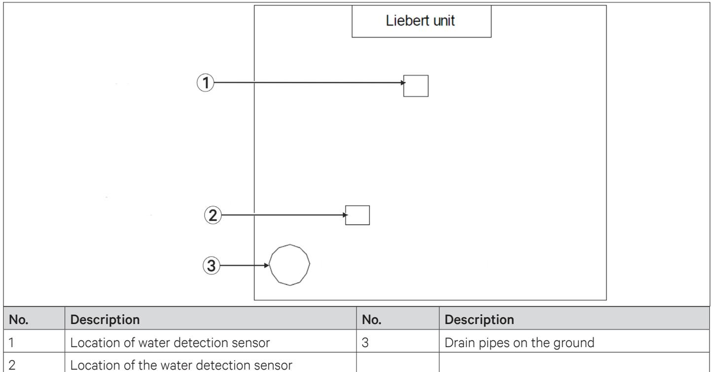
**Figure 4-1 Recommended Location for the Water Detection Sensor**
