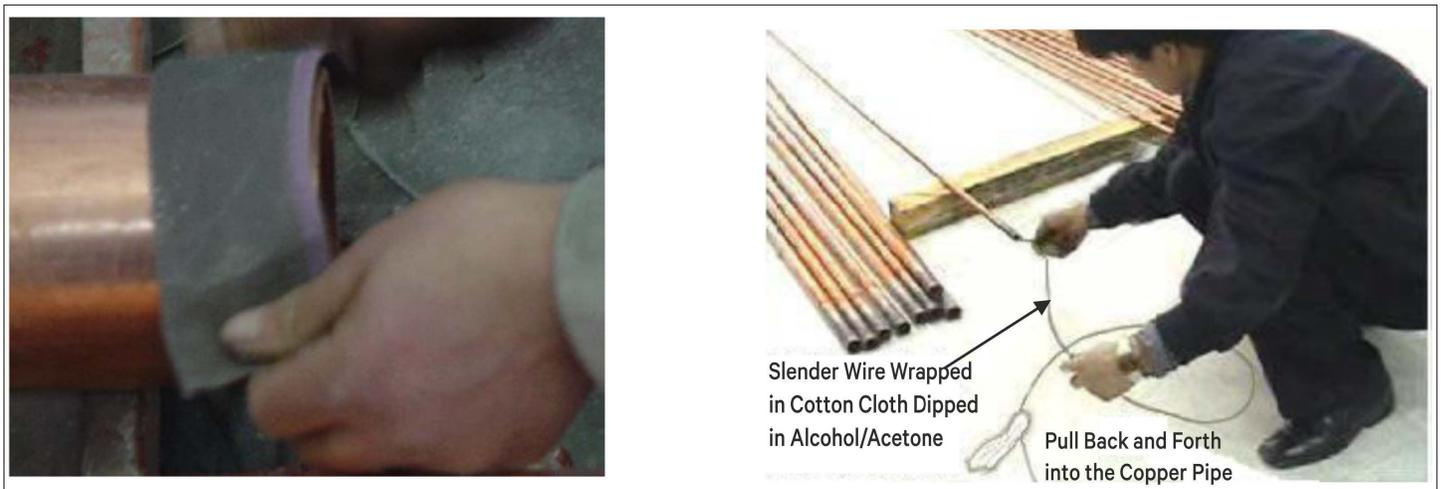
**Figure 2-21 Copper Pipe Cleaning Method**
