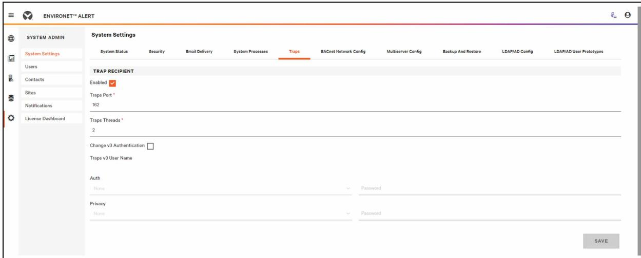
Figure 6.6 Trap Sender Setting
