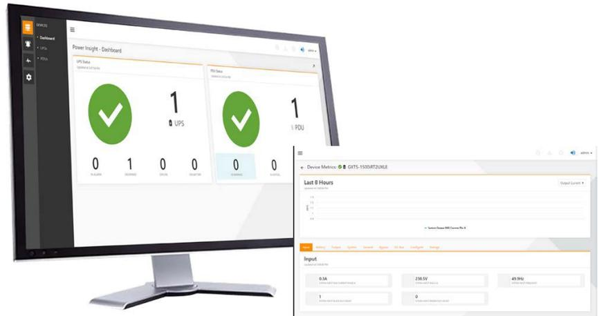
Organizations use Vertiv™ Power Insight to oversee the power solutions that support their distributed infrastructure. This complimentary, web-based software provides a single interface to monitor up to 100 Vertiv™ uninterruptible power supplies (UPSs) and rack power distribution units (rPDUs) and shut down critical computing resources.
