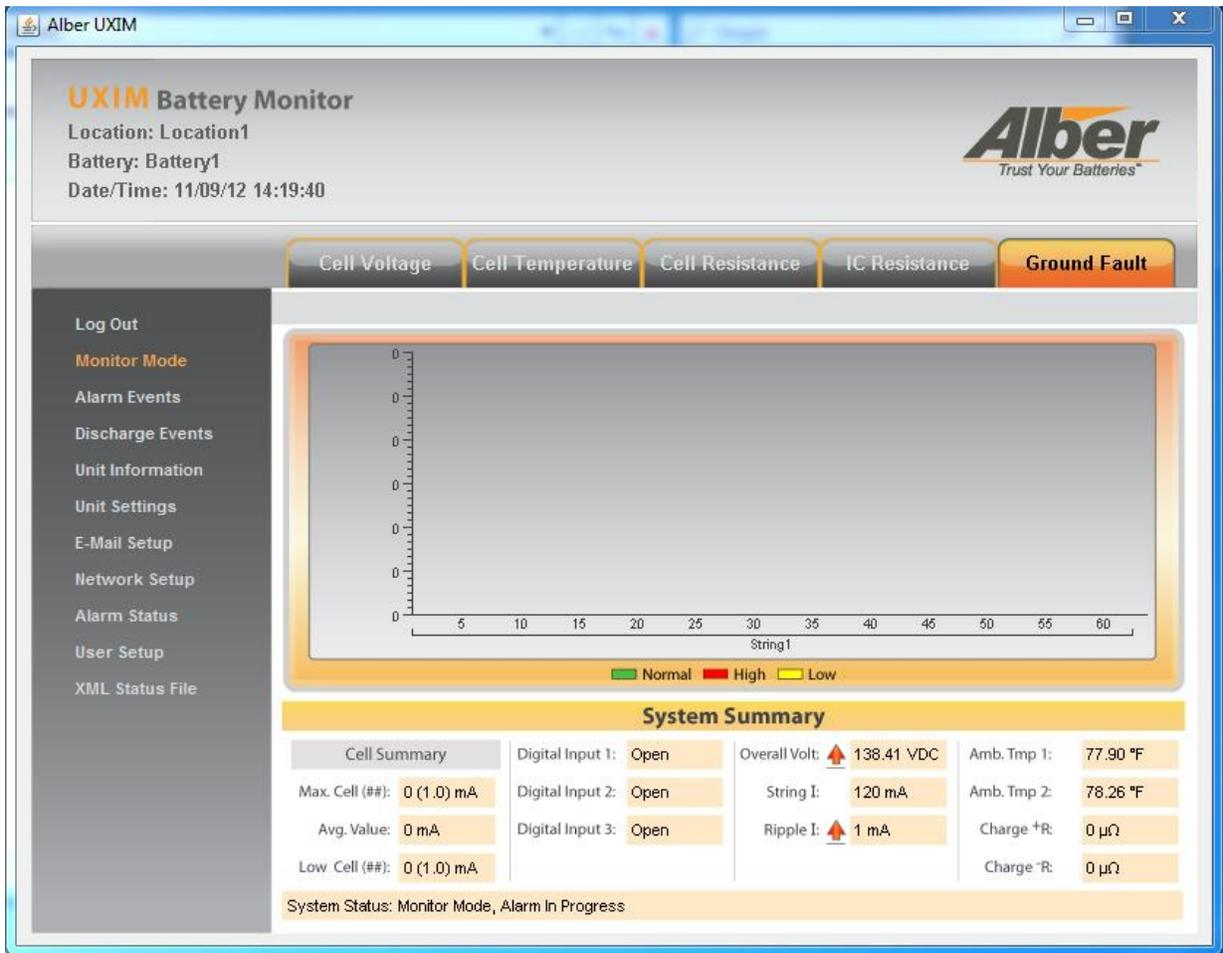
Figure 9 – Ground Fault Readings and Summary Information
