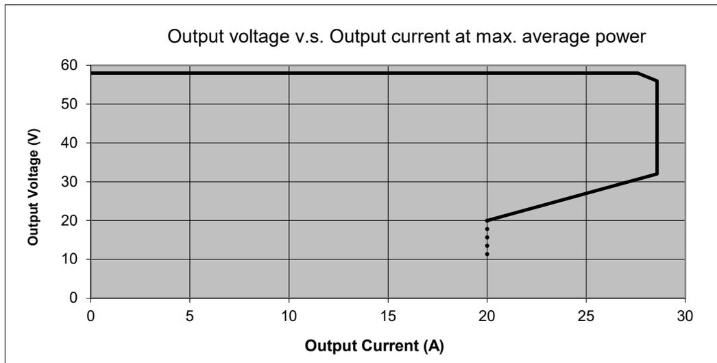
Figure 1.2: Output Voltage vs. Output Current at Maximum Peak Power 2000W
