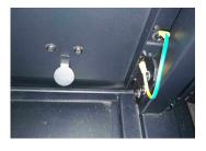
All rack panels and Doors are inherently grounded to Frame
