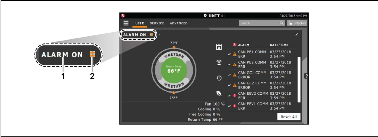
Figure 1.4 Unit Status on Liebert®iCOM™ Display
