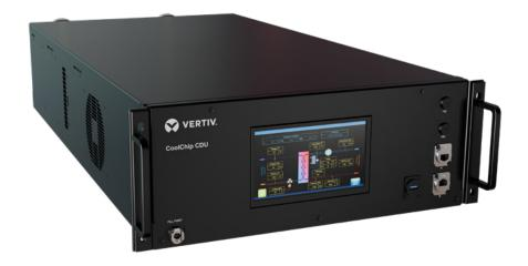
The Vertiv<sup>™</sup> CoolChip CDU 121 in-rack coolant distribution unit (CDU) provides effective separation of the facility fluid circuit and secondary fluid network via a liquid-to-liquid heat exchanger for single rack direct-to-chip cooling applications.
