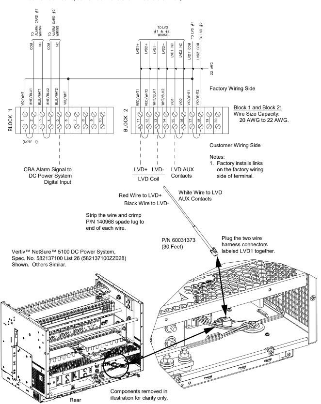
Figure 11.7 Typical Power System LVD Connections to Alarm BLOCK 2 (Vertiv™ NetSure™ 5100 DC Power System, Spec. No. 582137100 List 26, 582137100ZZ028 Shown. Others Similar.)
