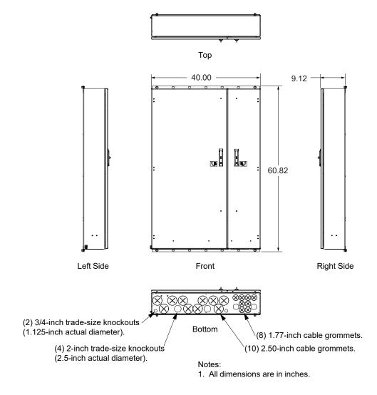
Figure 2.3 Enclosure Mounting Dimensions
