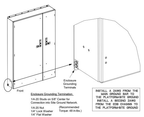
Figure 9.2 Enclosure Main Ground Bar Location
