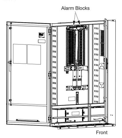
Figure 11.3 Alarm Block Connections - F1011259
