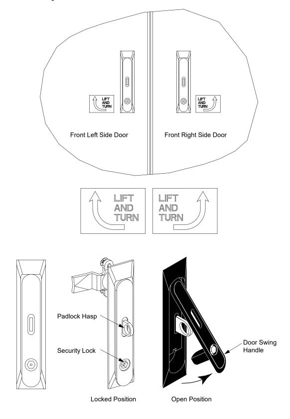
Figure 4.2 Enclosure's Left Side Front Door Wind Latch
