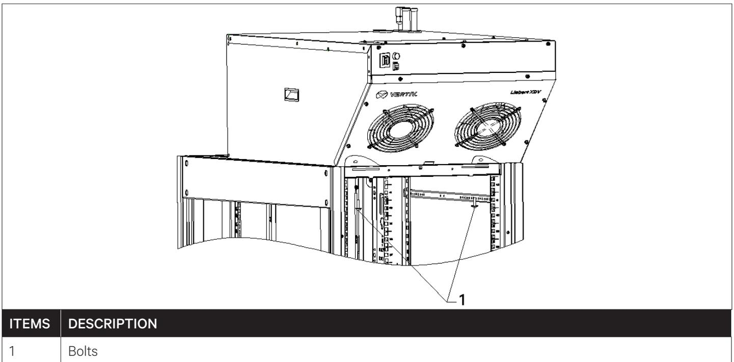
**Figure 2-10 Bolt Fixing the Cabinets and the Unit**
