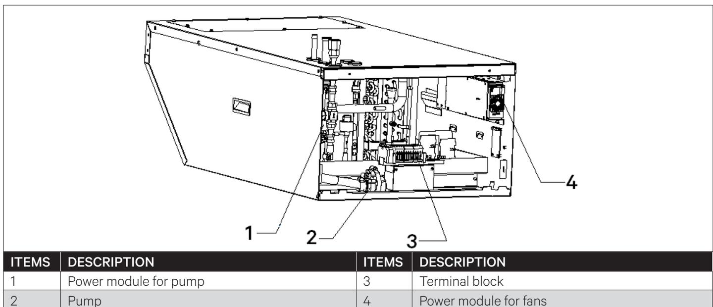
**Figure 3-2 Layout of the Rear Electric Control Box**
