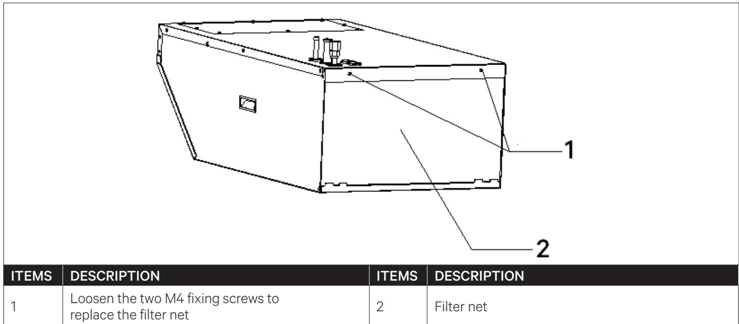
**Figure 3-1 Remove Filter Net**
