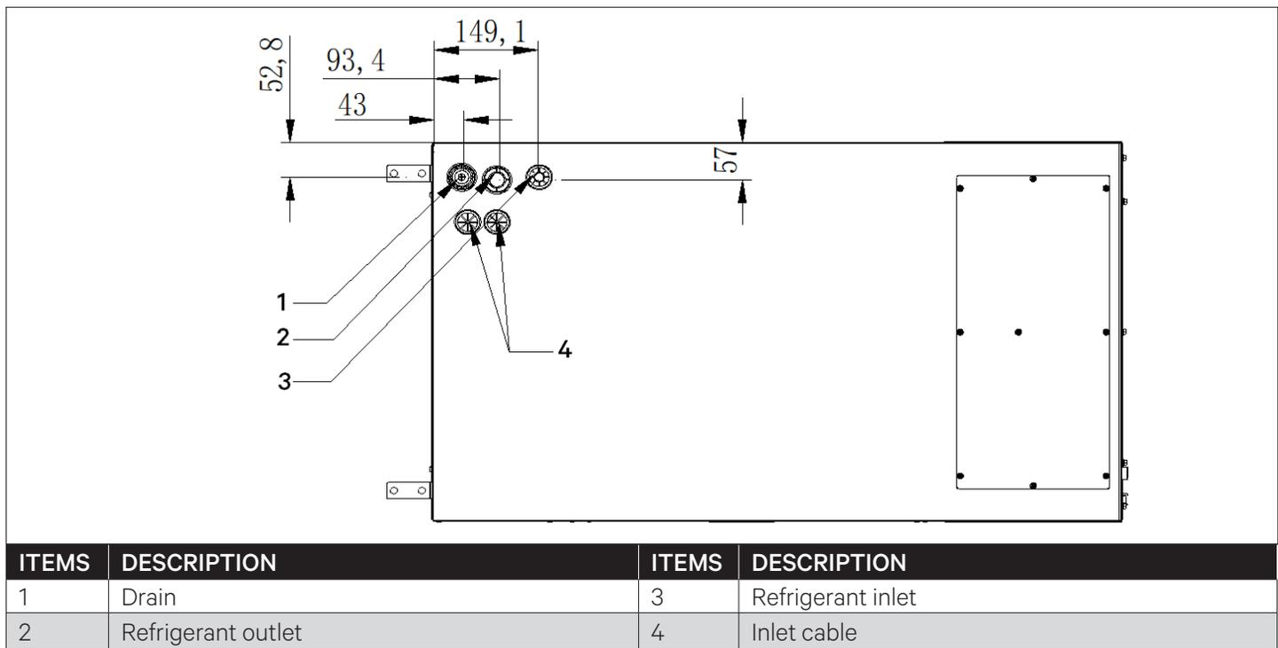
**Figure 2-7 Outlet Position of the Unit's Top Plate**
