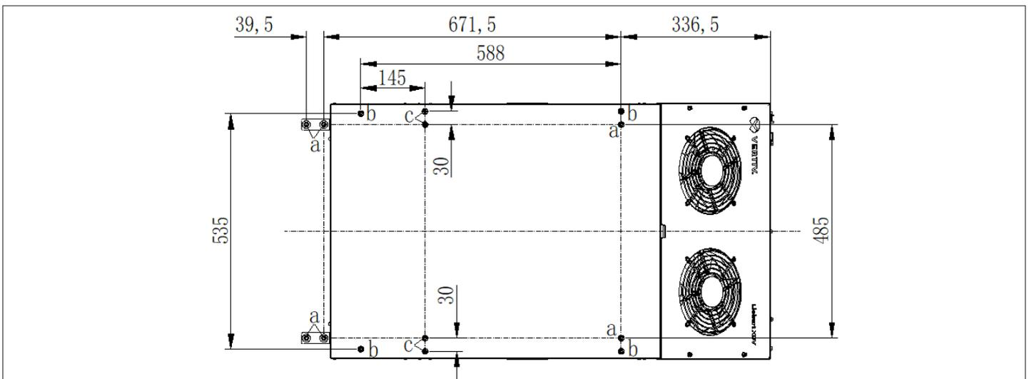
**Figure 2-12 Dimensions of Fixing Holes of the Unit**
