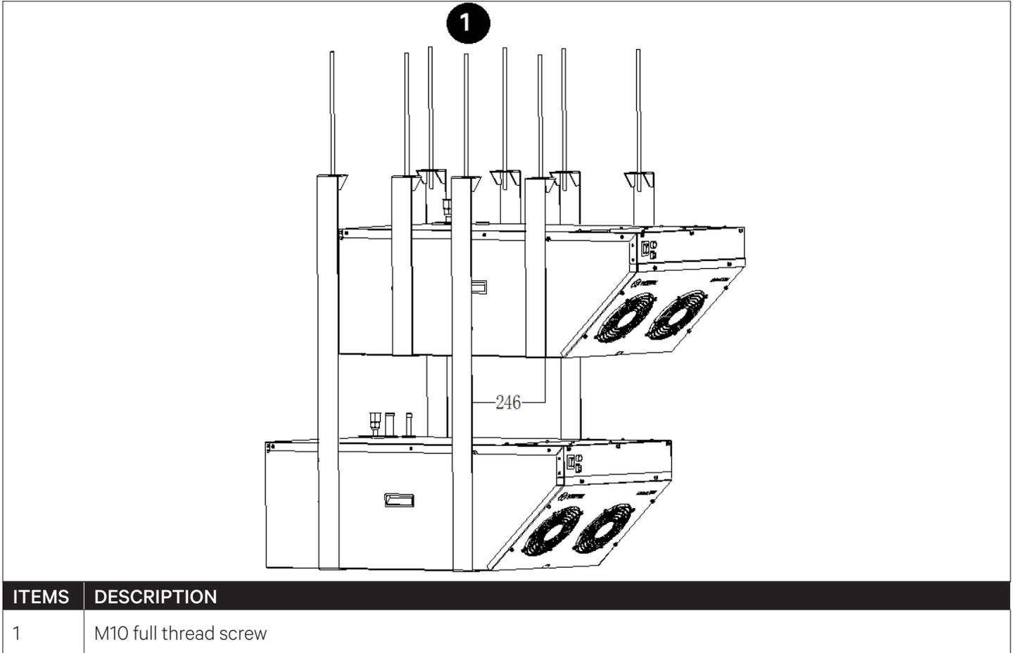
**Figure 2-19 Fixed Installation from the Ceiling and External Suspension**
