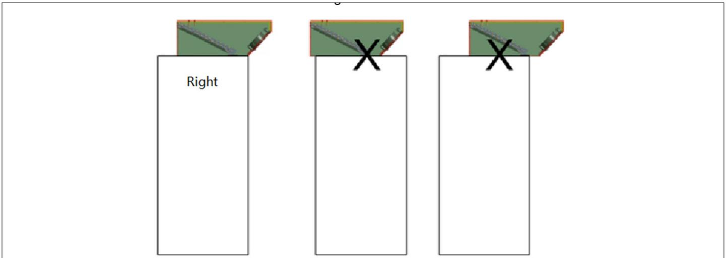
**Figure 2-9 Correct Installation Position of Unit**
