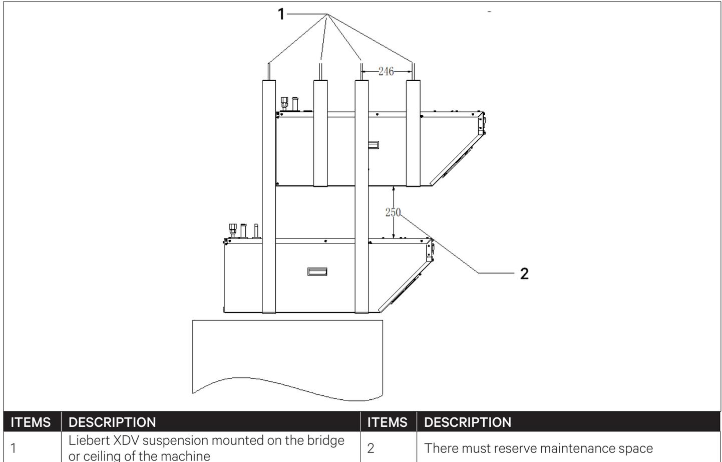
**Figure 2-16 Offset of Stacked Installation**
