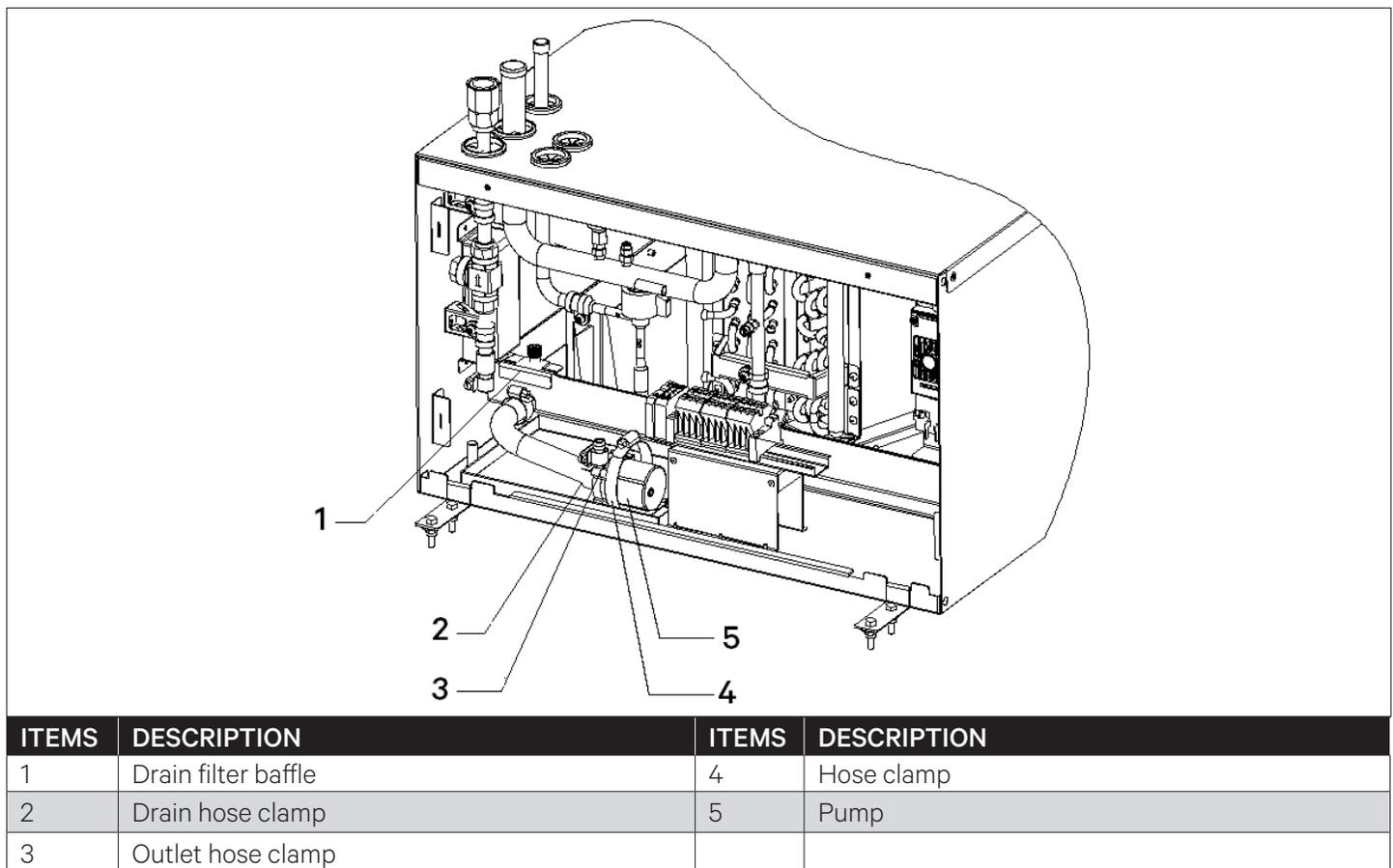
**Figure 6-1 Condensate Pump Removal**
