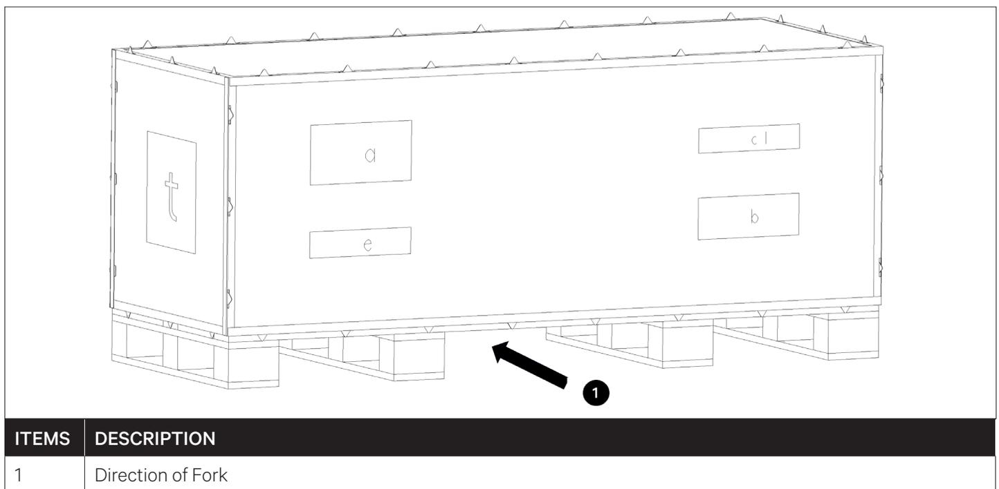
**Figure 2-2 Forklift Position to Lift the Unit**
