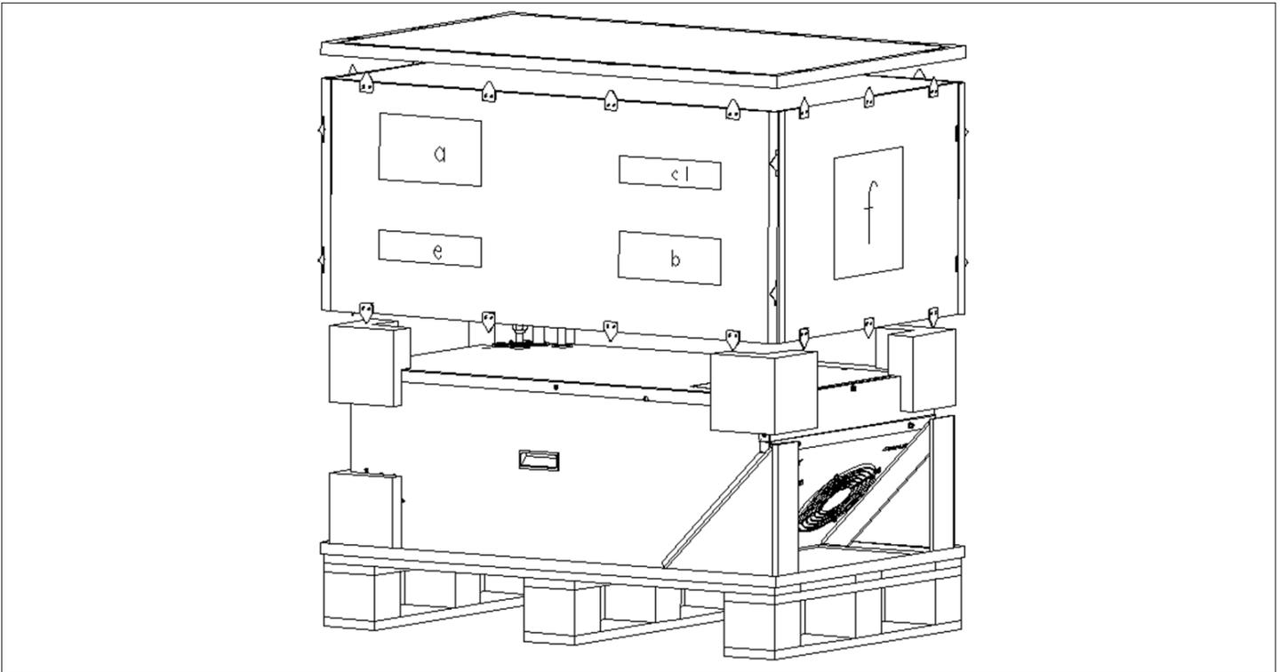
**Figure 2-4 Unpacking the Unit**
