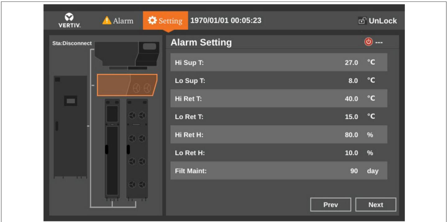
**Figure 5-11 Terminal Alarm Setting Interface**
