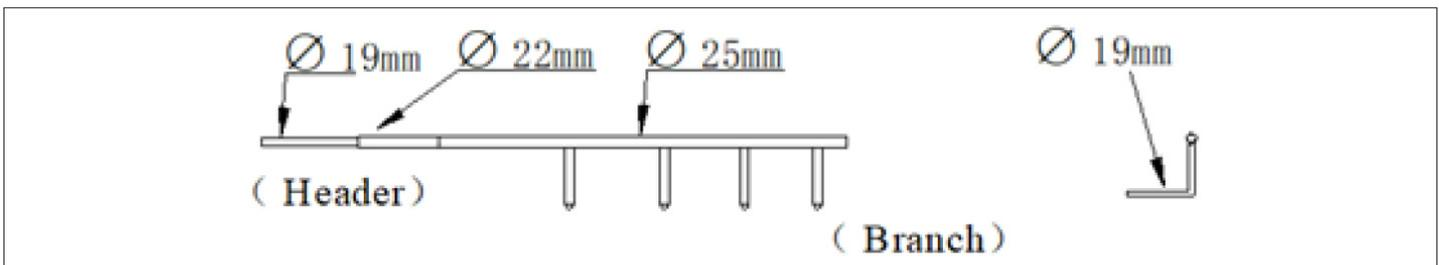
Figure 2-16 Branch Manifold of Liquid Return Pipe
