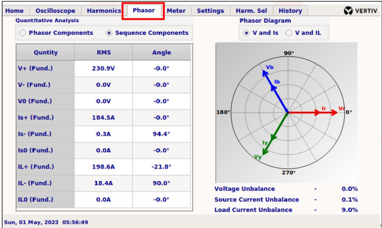
The Phasor tab does provide real-time phasor diagrams as well as sequence components analysis.
