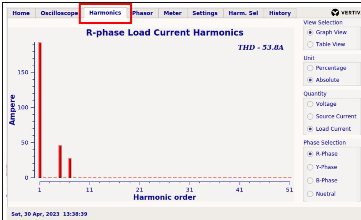
The Harmonics tab is designed for real-time analysis of individual harmonics present in the load as well as source current waveforms. The individual harmonics are shown in percentage with respect to fundamental current.
