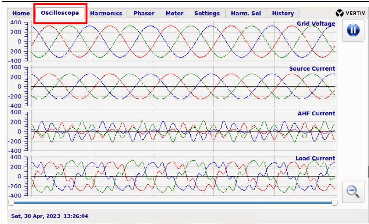
The Oscilloscope tab is equipped with 15 channel real-time oscilloscope, for graphical visualization of AHF performance in mitigating the current harmonics. The following waveform groups are displayed in real-time on Oscilloscope tab:
