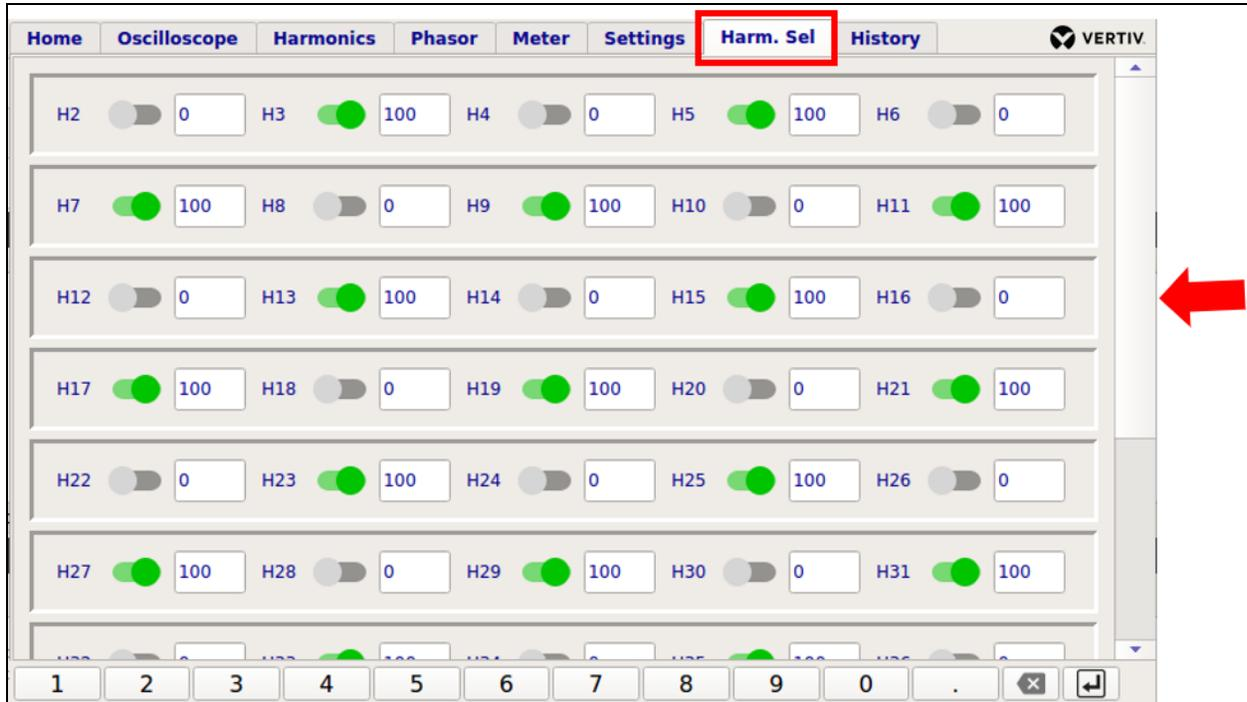
This screen allows the user to select or deselect the harmonic order to be compensated by the AHF. The selection/deselection can be made by switching ON/OFF the switch corresponds to harmonic order by a gentle touch on the toggle switch. There is no limitation on total number of harmonic orders that can be selected simultaneously for compensation. User can also enter the required percentage compensation for any selected harmonic order in the edit box corresponds to the harmonic order.
