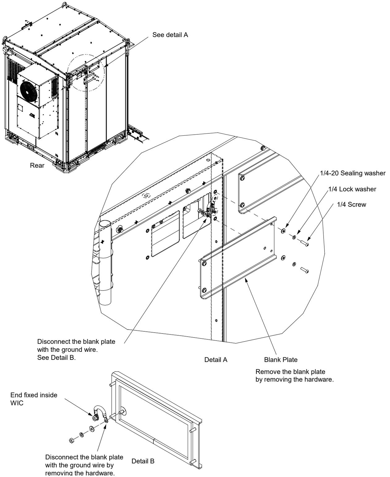
Figure 8.2 Installing the Wall Cable Port Plates
