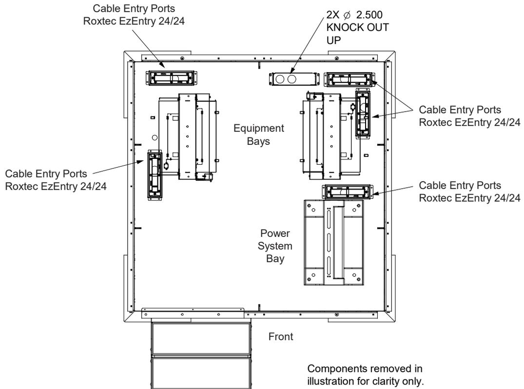
Figure 2.17 Wall Cable Entry Ports
