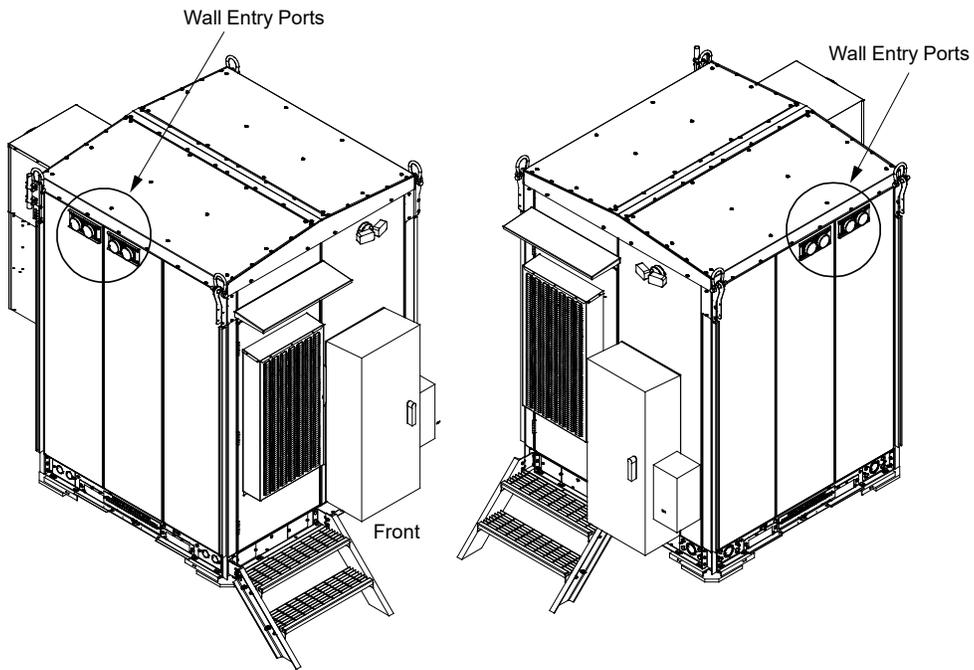
Note: 1. Port boots must be used to seal the cables.
