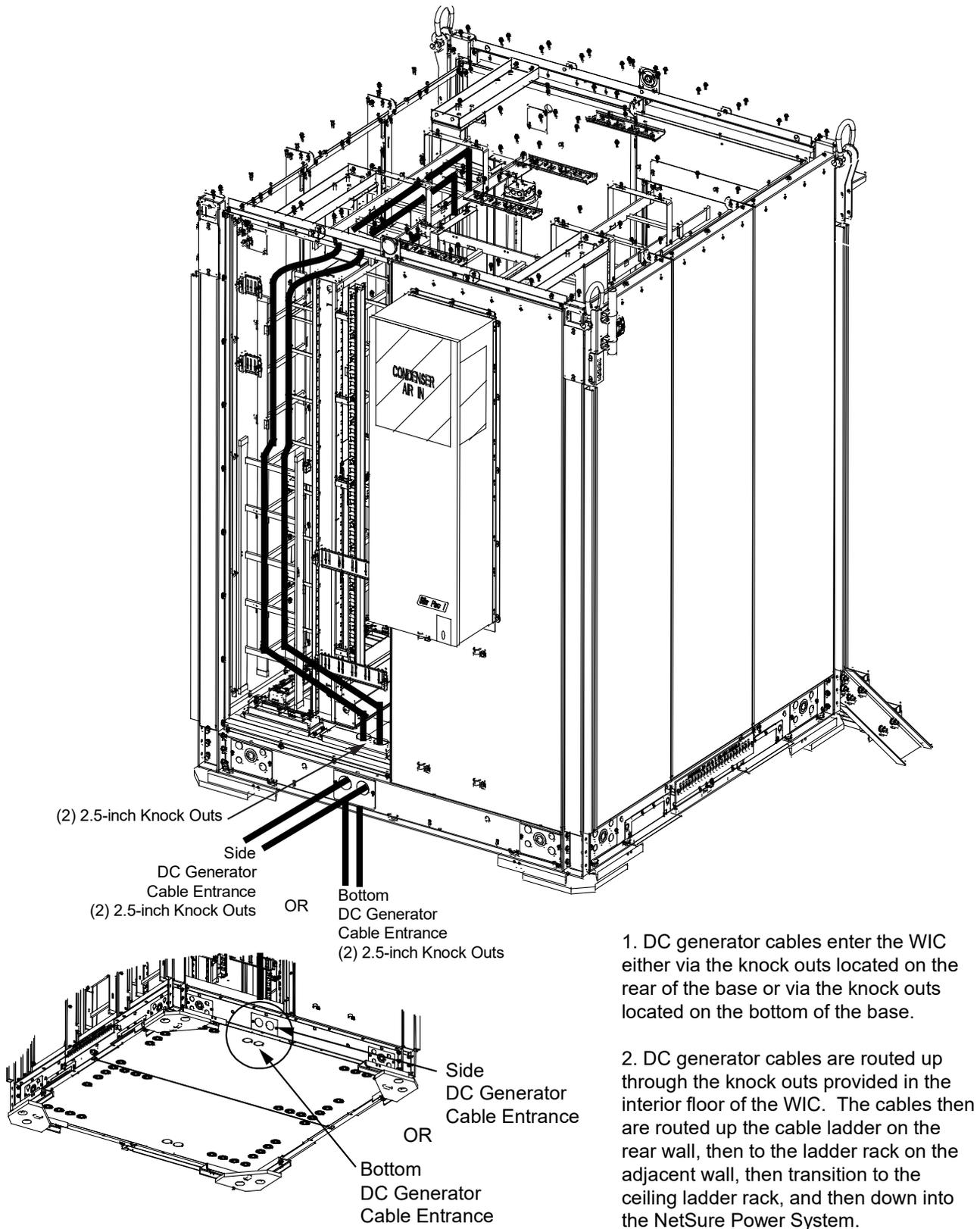
1. DC generator cables enter the WIC either via the knock outs located on the rear of the base or via the knock outs located on the bottom of the base.
