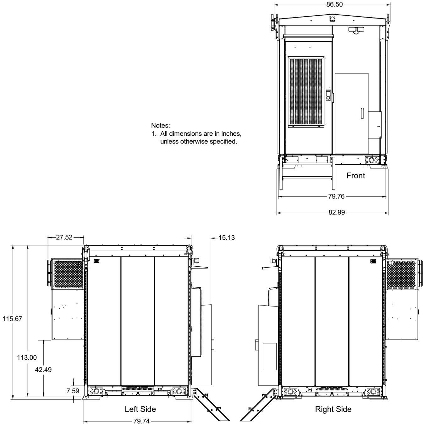
Figure 2.4 Mounting Hole Dimensions (with corner plates)
