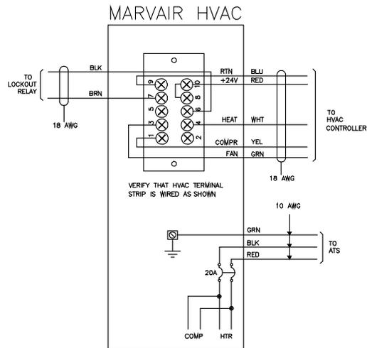
Figure 16.1 F2018009 Direct Air Cooling (DAC) and HVAC Schematic Diagram (cont'd from previous page)
