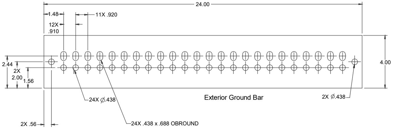
Figure 10.2 Typical Master Ground Bar Terminations (cont'd on next page)
