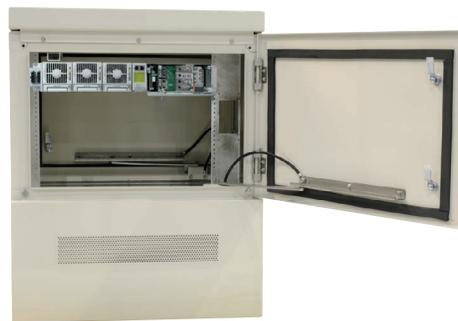
Heat exchangers, and fan/filters are controlled by the Vertiv XTE 601 Cabinet Controller that turns fans on and off to maintain equipment chamber temperature within designated limits. It also reduces fan speed at low load or low ambient temperature to reduce power consumption and minimize acoustic noise. The controller reports fan failures and extreme high and low temperatures as alarms. The controller also monitors door intrusion alarms (remote and audible).
