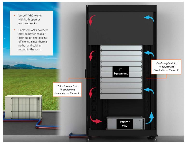
Airflow Diagram Vertiv<sup>™</sup> VRC
