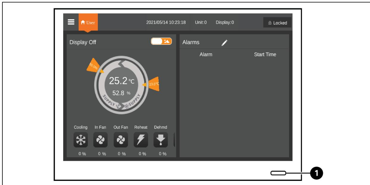
The indicator (1) is located under the screen. Its colors and indication are described in **Table 7.11** below.
