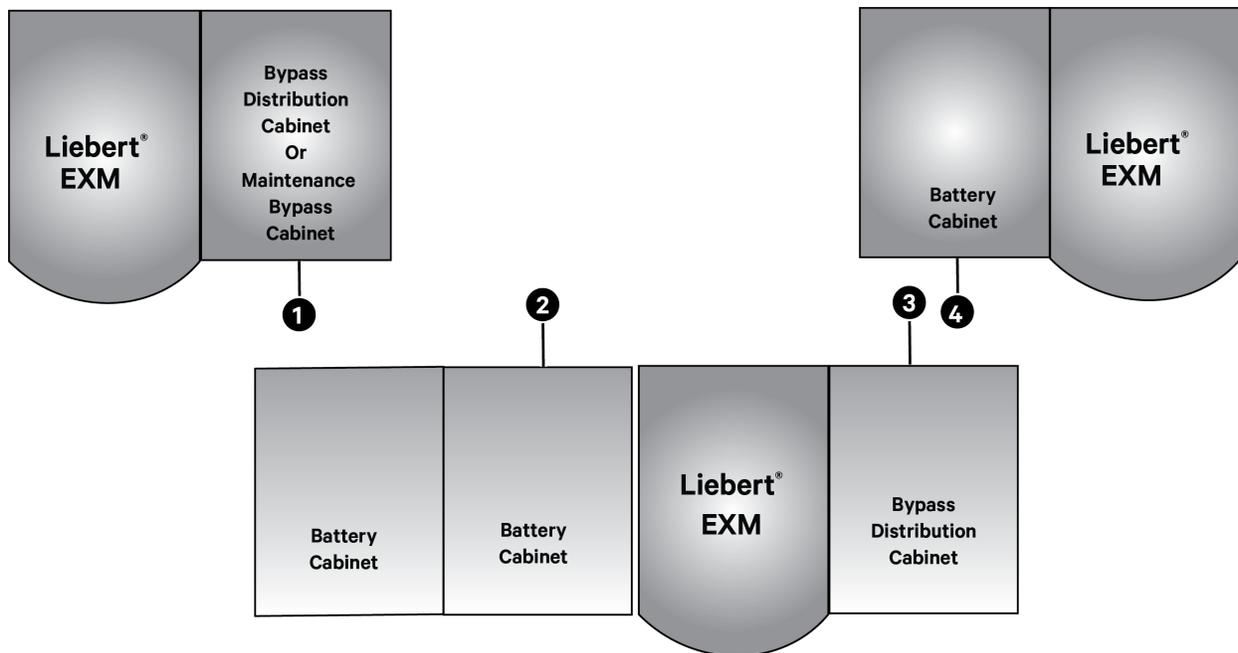
**NOTE: All the units viewed from above. layouts shown are typical. not all auxiliary cabinets are shown. Refer to the submittal drawings for the exact configuration of your system.**
