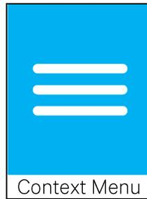
Parallel operation differs depending on the software in the control menu. To determine which version is installed on the UPS, activate the touchscreen menu, touch the Context Menu and touch About.
