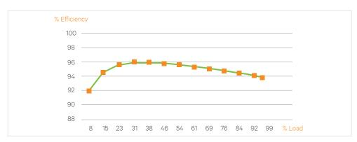
eSure Converter Efficiency Curve
