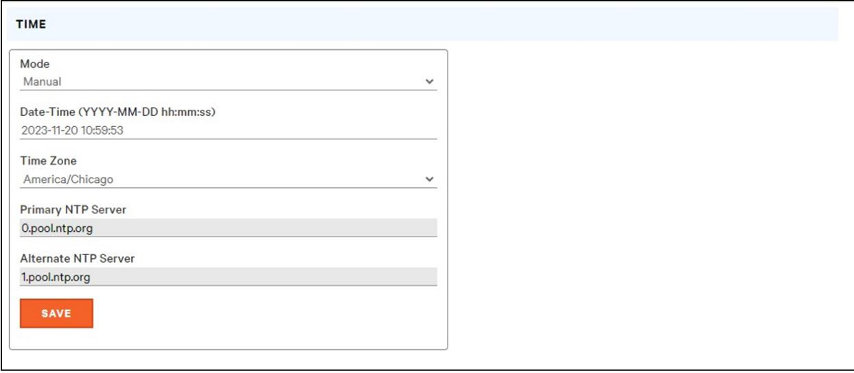
The screenshot shows a configuration page titled "TIME". It contains several fields: "Mode" is set to "Manual"; "Date-Time (YYYY-MM-DD hh:mm:ss)" is "2023-11-20 10:59:53"; "Time Zone" is "America/Chicago"; "Primary NTP Server" is "0.pool.ntp.org"; and "Alternate NTP Server" is "1.pool.ntp.org". A red "SAVE" button is located at the bottom left of the form area.
