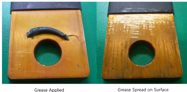
Figure 3-49: Conductive Grease on Busbar
