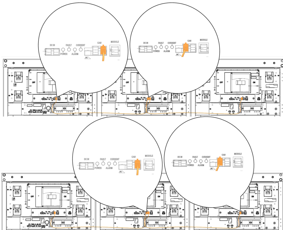
Figure 3-123: BCU-to-BCU Signal Cabling Connection Examples (System BMS on the left)
