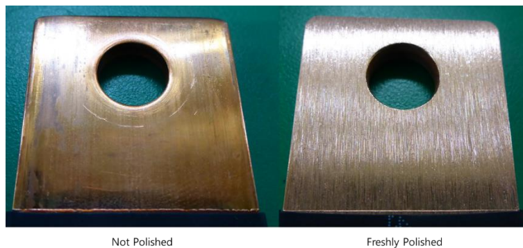
Figure 3-48: Copper Busbar Appearance
