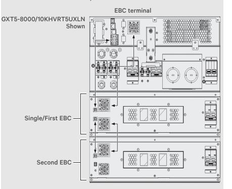
**GXT5 UPS to External Battery Cabinet Connections**
