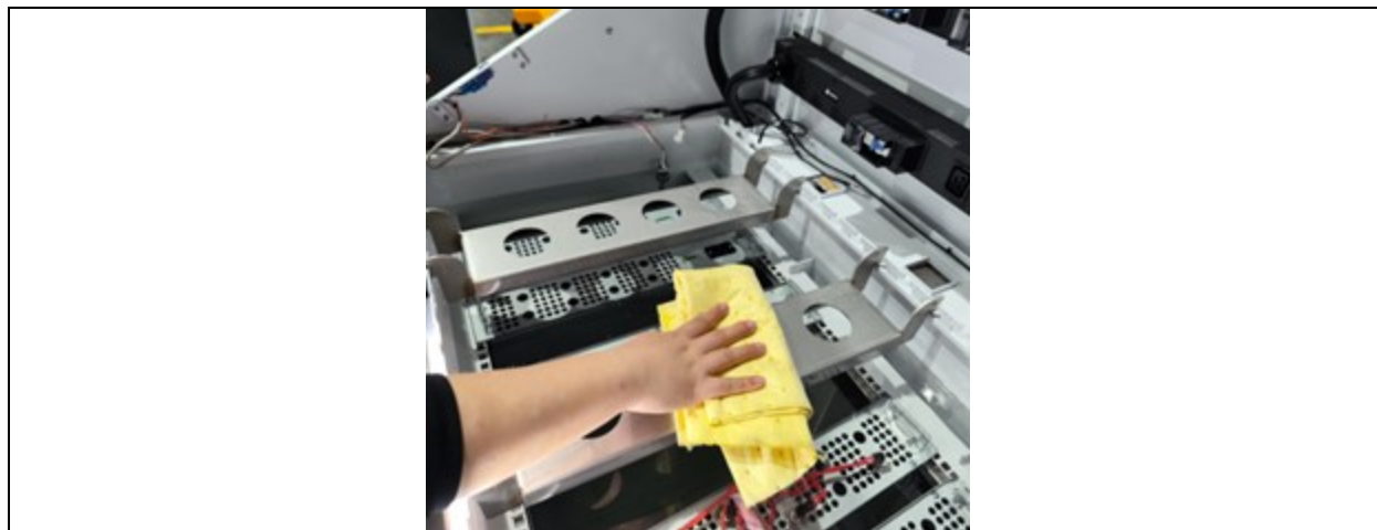
Figure 7.10 Wiping the guide rail
