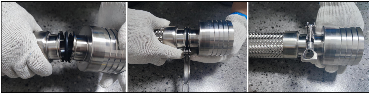
Figure 4.15 Connecting the Grooved Clamp
