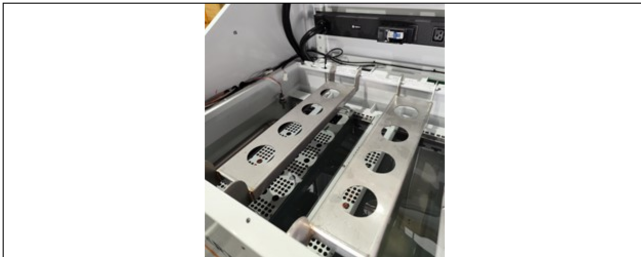
Figure 7.6 Placing the guide rail
