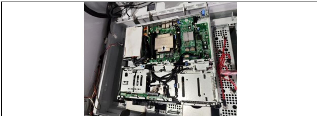
Figure 7.9 Placing the server on guide rail
