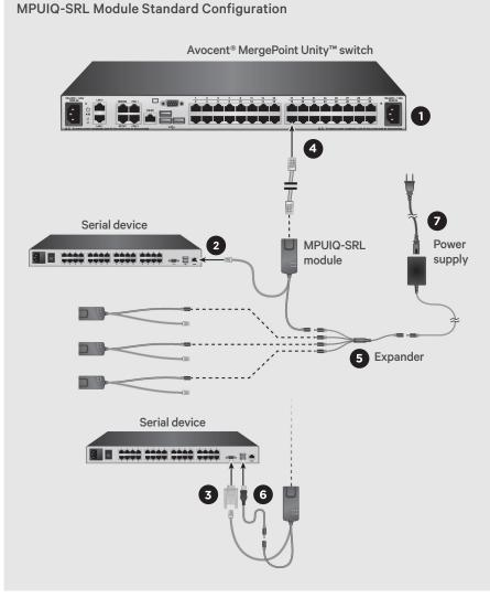
MPUIQ-SRL module. Plug the other end into the USB port on your serial device.
