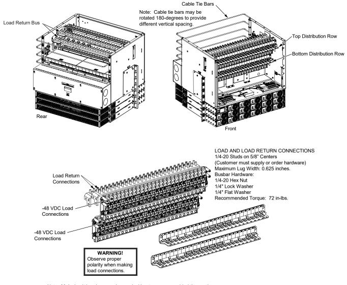
Note: 80 A circuit breakers can be used without a space provided the continuous current in each 80 A device does not exceed 51 A. A 100 A or greater circuit breaker SHALL HAVE an empty mounting position between it and any other overcurrent protective device.
