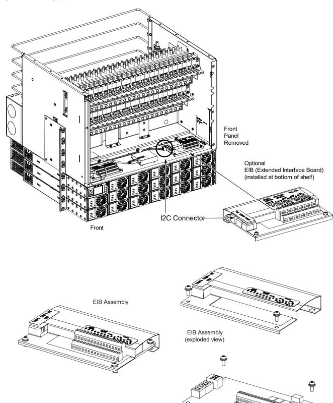
Figure 3.3: Installing Optional EIB (Controller Extended Interface Board)
