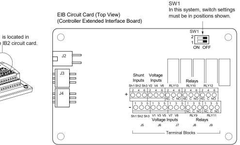
Switch SW1 is located in this corner of the IB2 circuit card.
