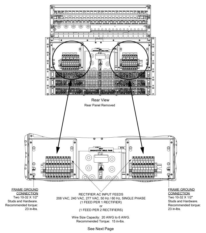
Figure 5.2: AC Input Connections to AC Input Termination Assembly (Nominal 208 VAC, 240 VAC, 277 VAC) (1 Feed per 1 Rectifier, Single Phase or 1 Feed per 2 Rectifiers, Single Phase) (cont'd on next page)
