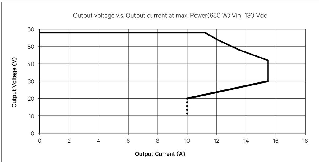
**Figure 1.3 Output Voltage vs. Output Current with DC input(810W)**
