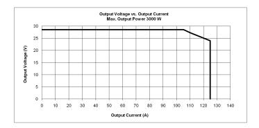
Power Derating Based on Input Voltage: The rectifier can provide maximum rated power (2500W or 3000W) as long as the
